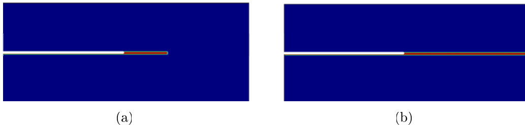
Figure 5.12. The final crack path of the element deletion method with a 200 \times 81 structured quadrilateral mesh at different time steps: (a) t = 30.56 \mu\text{s} and (b) t = 65.62 \mu\text{s} .
