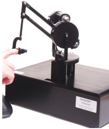
Figure C.4. The PHANTOM device for haptic interaction (photo courtesy of SensAble Technologies).
