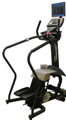
Figure C.1. The haptic robotic stair climber created by me, Ferber, and our colleagues at Northwestern University. [43]
