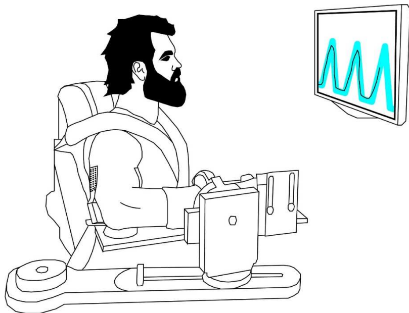
Figure 5.1: Illustration of the experimental setup. High-density surface electromyography (HD-sEMG) arrays were placed on the lateral head of the TRI and along the muscle belly of the BIC.
