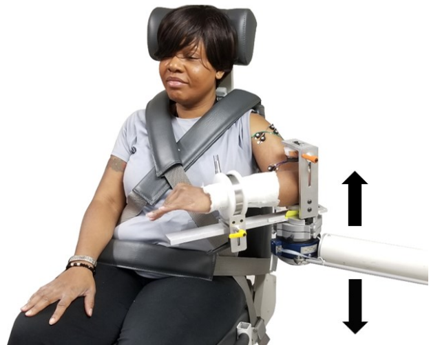
Figure 22. Participant set up in the ACT 3D robot. Humeral abduction angle reduced for visual appreciation. Robot is controlled via force or position but only in the vertical direction (denoted by arrows) via online classifier. Shoulder internal and external rotation are fixed at anatomical neutral. All other motions at the shoulder and elbow are free and controlled solely by the participant.
