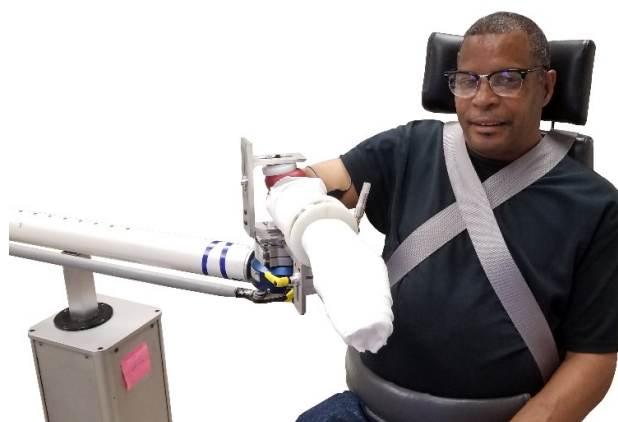
Figure 9. Dual-task setup. Custom ACT 3D with load cell (in blue under elbow) with casted arm attached via custom device. Movement of the robot was limited to the vertical direction. This participant's arm is resting on lower horizontal surface.
