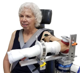
Figure 19. Participant in setup. Robot arm extends toward bottom right. Entire arm is able to abduct (up) and adduct (down) 2 inches in either direction. Forearm is held via rigid cast.
