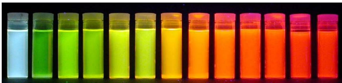
**Figure 3.2.** Fluorescence image of CdSe quantum dots showing an increase in QD size going from blue (~1 nm in diameter) on the left to red (~5 nm in diameter) on the right.
