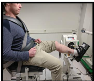
**Figure 1.** Isometric joint torque recording device with high-density surface EMG grids on the soleus and tibialis anterior muscles.
