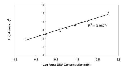
Figure 7: Preliminary results for standard Alexa-labeled DNA curve showing a linear relationship between Alexa-labeled DNA and emission area from picomolar to nanomolar range.
