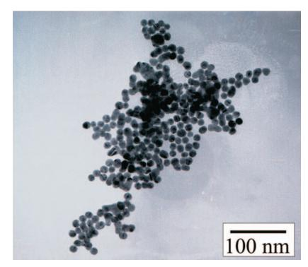
Figure 4: A TEM image of 13 nm gold particles emphasizes size and spherical shape.
