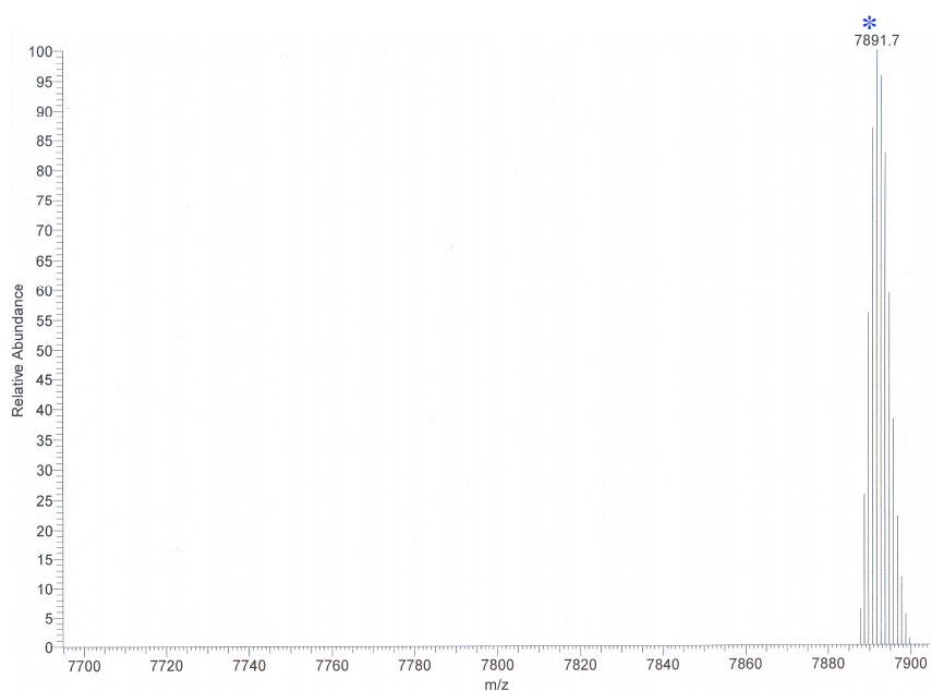
Figure 6.10 ESI-MS spectrum of protein band # 8 (*) (RT: 11.38 min) [apo-Cc2a: m/z^{\text{calc}} = 7882.9 (red), m/z^{\text{calc}} = 7880.9 (oxid), m/z^{\text{obs}} = 7891.7 ].
