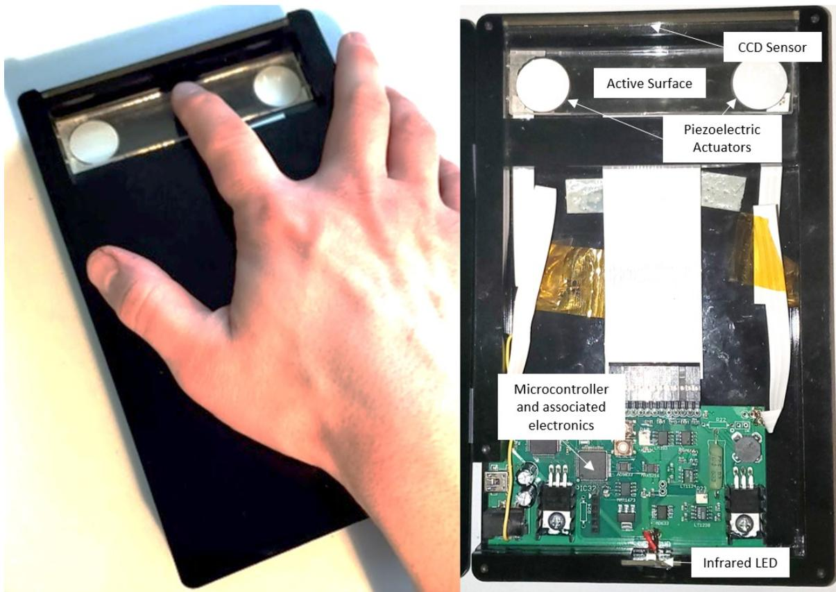
Figure 2.1. High-Performance TPaD surface haptics device
