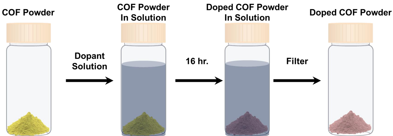
Figure 11.12. Illustration of the general doping protocol.
