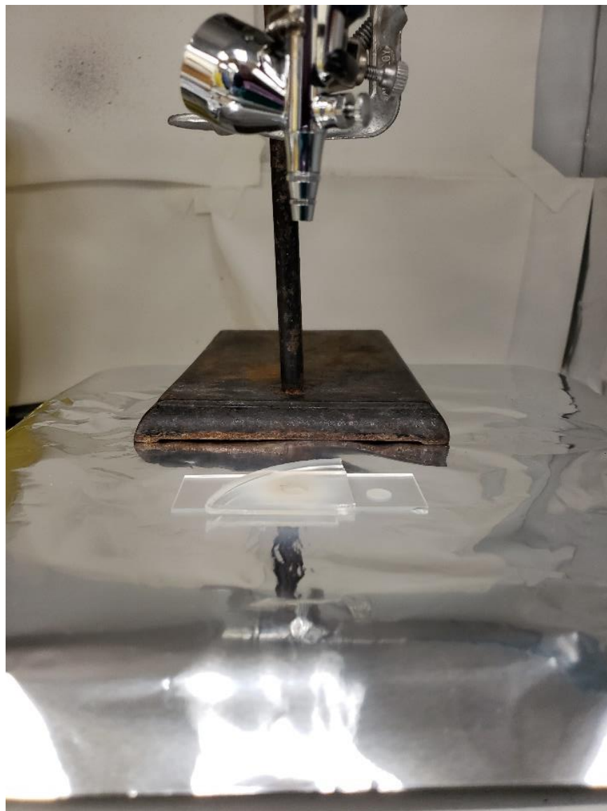
Figure 8.60. Image of COF printing setup.
