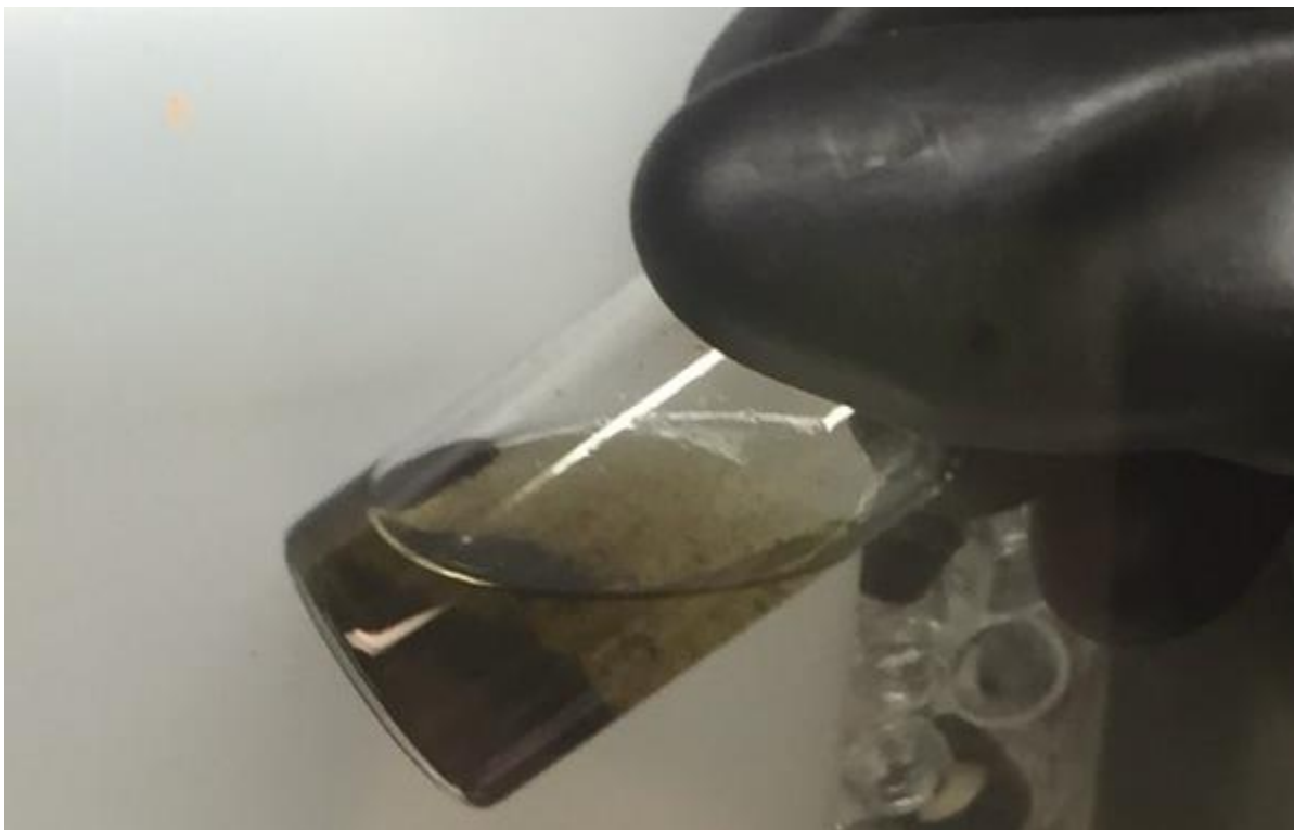
Figure 11.14. Representative photograph of molecular reduction of NDI-based COFs. Dark COF powders have settled to the bottom of the vial and the supernatant is now yellow, consistent with the oxidation of \text{CoCp}_2 to \text{CoCp}_2^+ .
