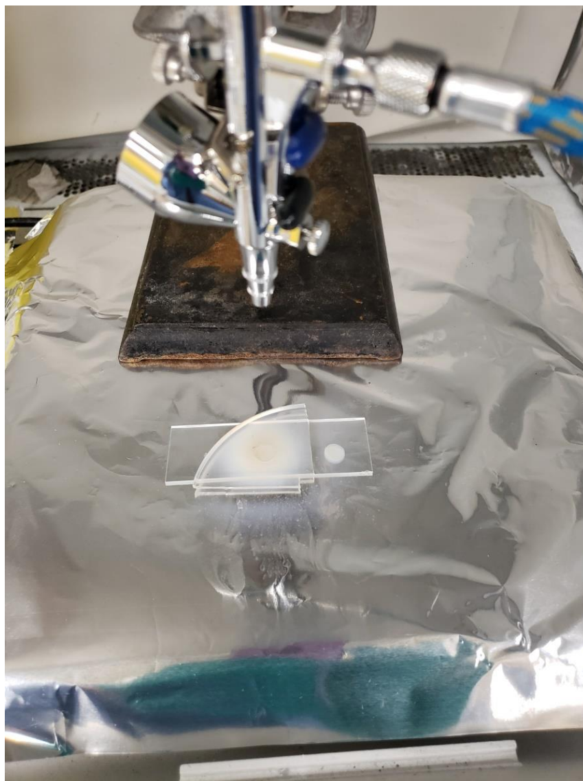
Figure 8.61. Image of COF printing setup.
