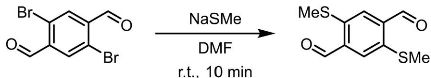
Scheme 6.8. Synthesis of 2,5-bis(methylthio)terephthalaldehyde ( S8 ).
