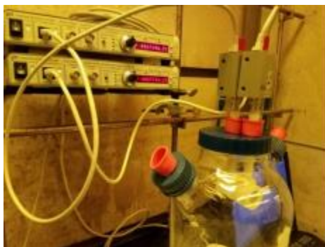
Figure 8.62. Image of QCM chamber used for COF sensing measurements.
