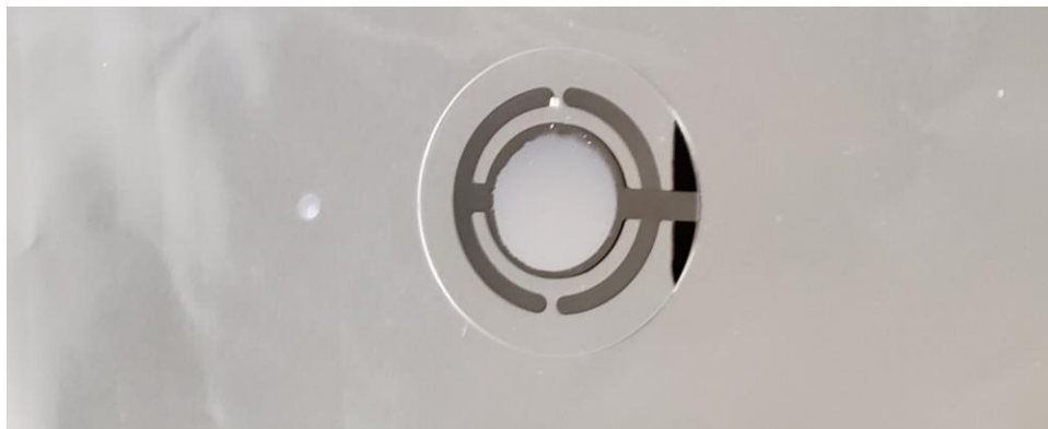
Figure 8.59. Optical image of spray-coated COF-10 on a QCM wafer.
