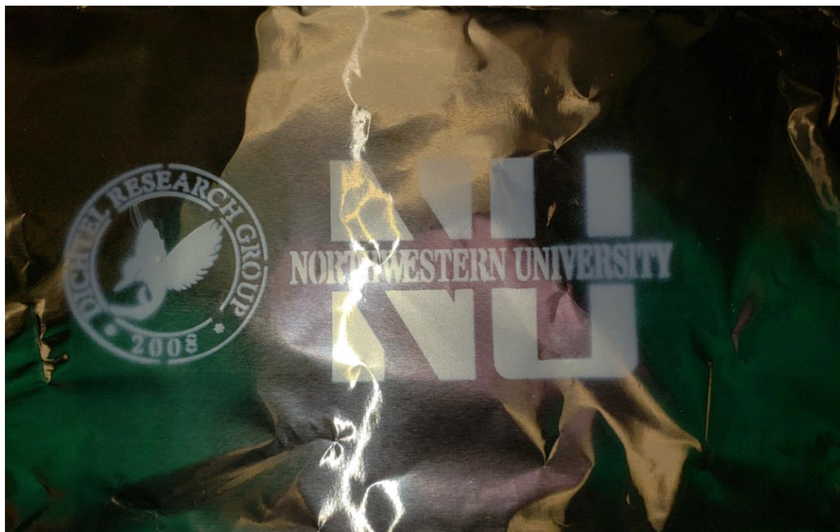
Figure 8.28. Optical image of printed logos on aluminum foil.
