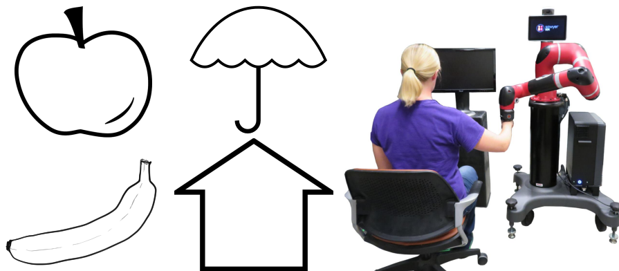
Figure 5.1. Participants were seated in front of a display showing the reference image and corresponding square in which they were to copy the drawing. They held onto a handle rigidly fixed to the end-effector of the Sawyer robot. The display provided visual feedback on what they had drawn so far and the amount of time remaining. A physical card with the given reference image was displayed throughout each trial. Study participants were asked to reproduce the images on the left as quickly as possible. They were given a maximum of 10 seconds per drawing.
