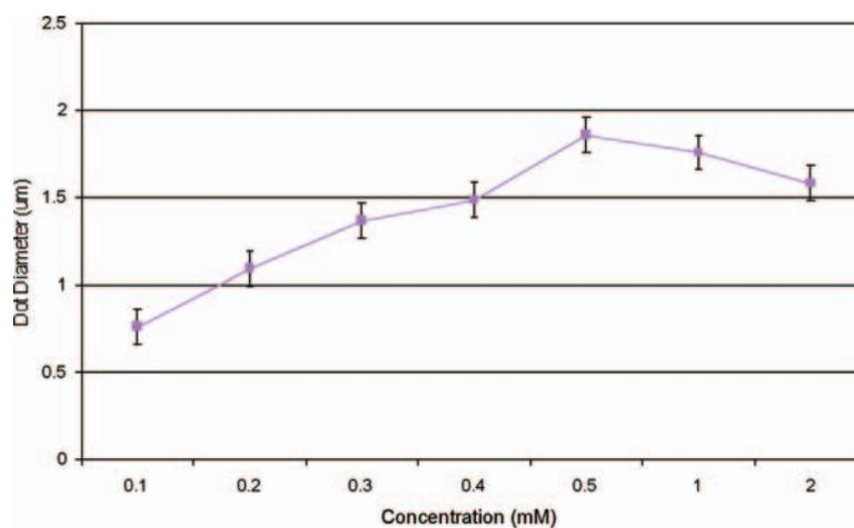
Figure 7: Dot diameter vs. concentration for contact time of 150 seconds.
