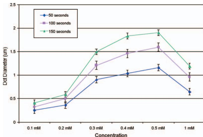
Figure 5: Dot diameter vs. concentration for three contact times (23.0° to 23.6° C, 59 to 62 percent humidity).
