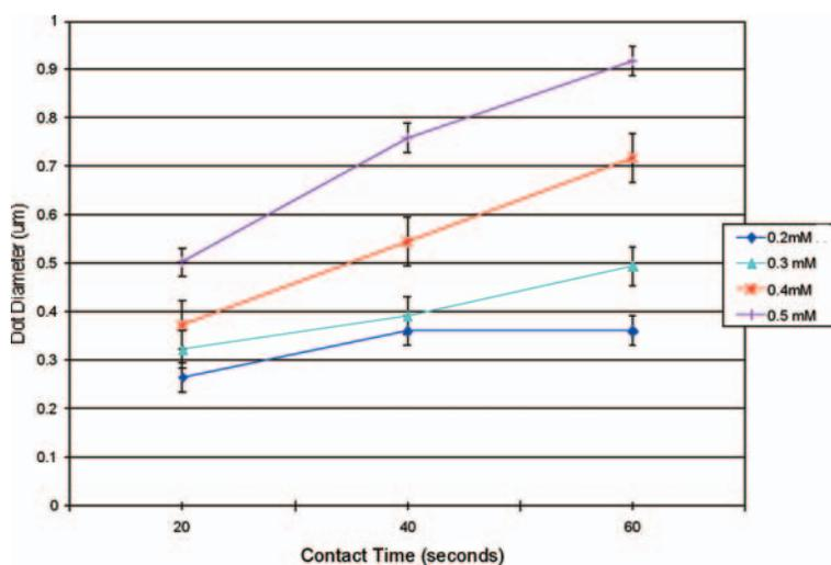
Figure 4: Dot diameter vs. contact time for 20, 40, and 60 seconds (22.0° to 22.9° C, 57 to 62 percent humidity).
