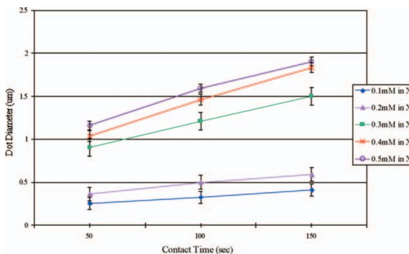
Figure 3: Graph of dot diameter vs. contact time for 50, 100, and 150 seconds (23.0° to 23.6° C, 59 to 62 percent humidity).
