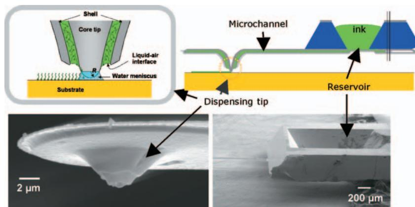
**Figure 1:** Diagram and SEM images of nano fountain probe. The image in the upper left corner shows deposition of ink (represented in green), while the image at the upper right illustrates the spatial relationship between the ink reservoir and the dispensing tip.
