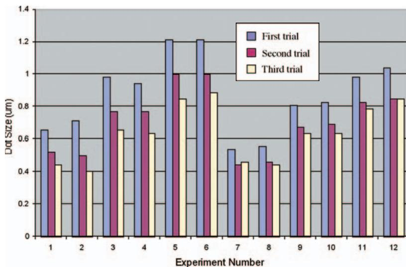
Figure 8: Dot diameter across three trials for 12 different experiments (0.5 mM, 20.9° to 21.7° C, 61 to 65 percent humidity).
