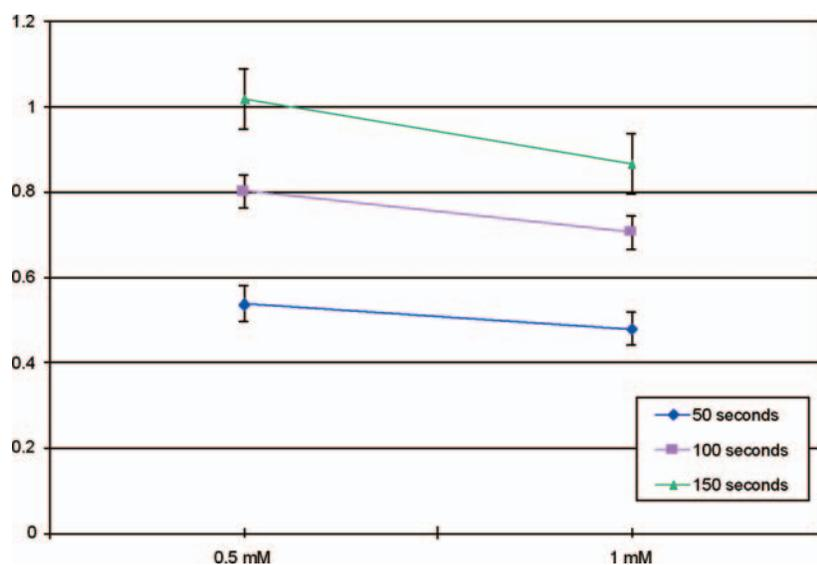
Figure 6: Dot diameter vs. concentration for three contact times (20.5° to 20.9° C, 64 to 67 percent humidity).
