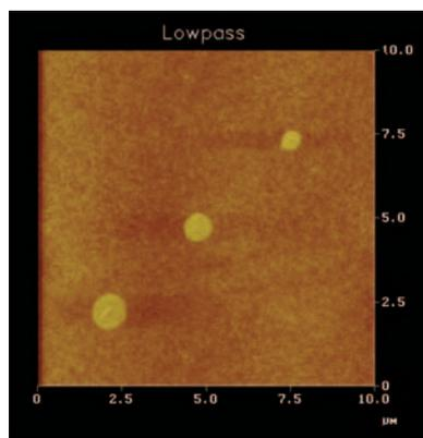
**Figure 2:** Lateral force image of patterned dots after dip-pen nanolithography has been performed with MHA molecules on an Au substrate (10 $\mu\text{m}$  x 10 $\mu\text{m}$ ).
