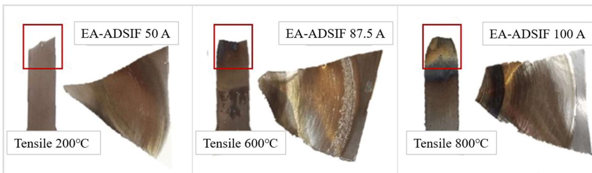
Figure 4.17 Color comparison between the samples obtained from the tensile and EA-ADSIF tests. The red box represents the area heated by the induction heating system during the tensile tests.
