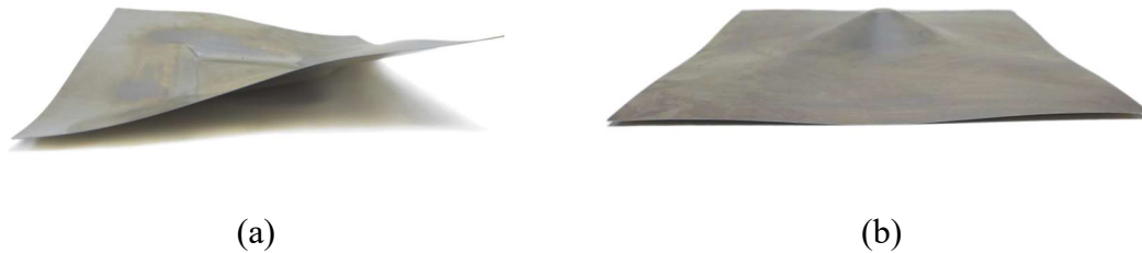
Figure 3.5 Formed parts after releasing from the clamps: (a) pyramid; (b) cone
