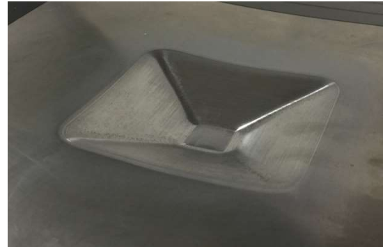
Figure 4.21 Ti6Al4V pyramid part using EA-MDSIF 50 A : (a) desired part; (b) formed part
