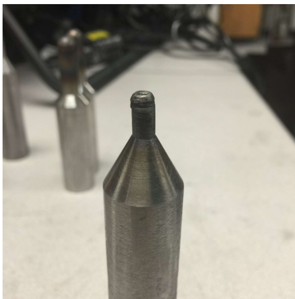
Figure 6.17 Severe damage of A2 tool steel tool after one EA-ADSIF 120 A process
