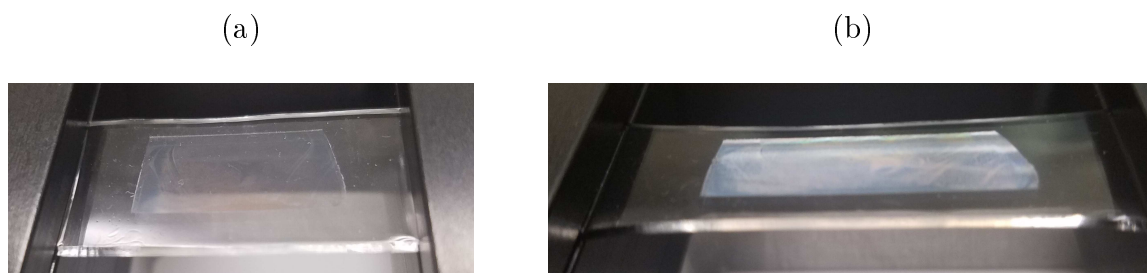
Figure 6.4: Polycarbonate thin film transferred to a clamped slab of PDMS (a) before testing and (b) during testing.
