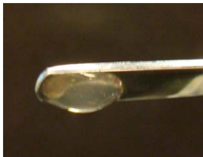
Figure 7.3.4: Photograph of self-assembled hydrogel formed by (BASE-K8 15 ) 2 at 15 wt% in H 2 O.
