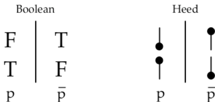
Figure 6: A comparison of the truth table for Boolean NOT and heed NOT operators
