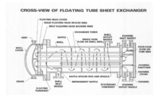
Figure 5: Shell and Tube Heat Exchanger (regonline.com)
