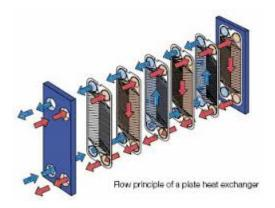
Figure 7 : Gasketed-Plate Heat Exchanger (wassertech.com)
