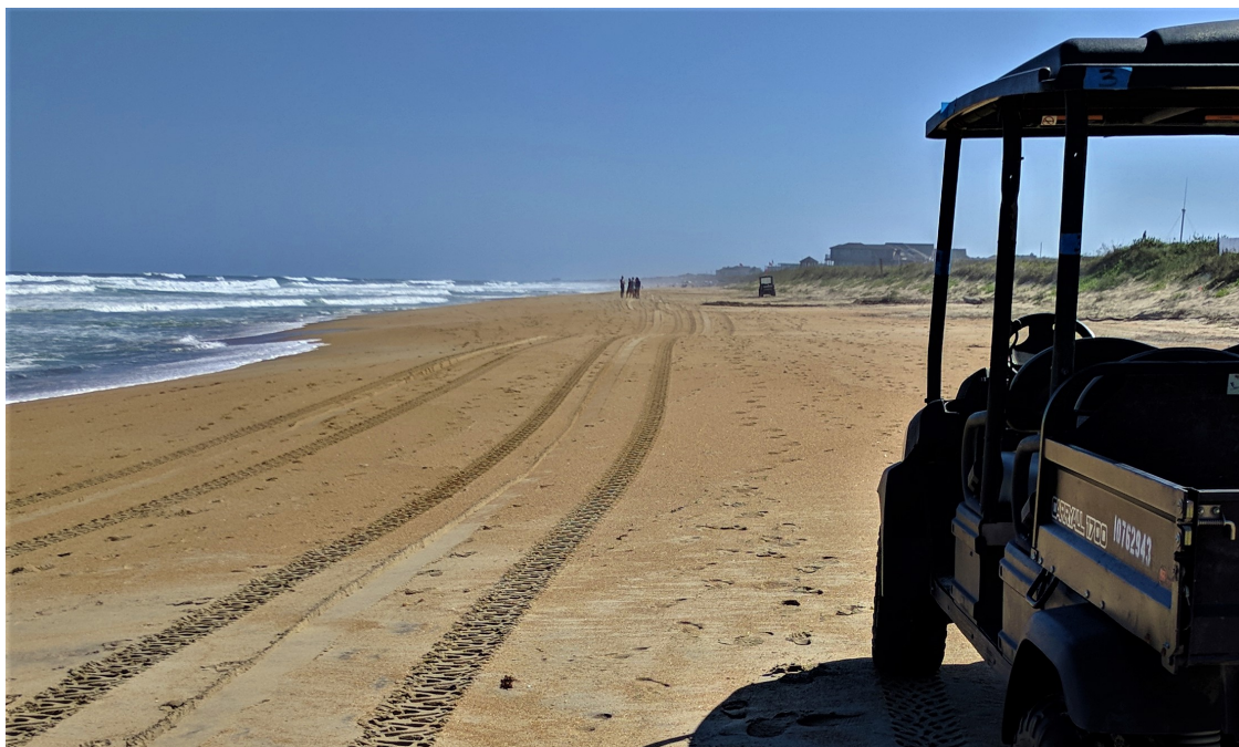
Figure 5.2: Beach with rut produced by tow test, visible between wheel tracks left by vehicle.
