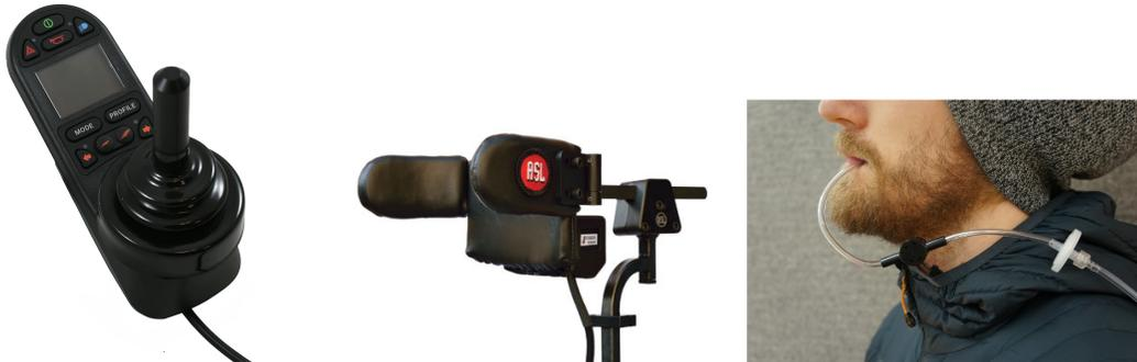
Figure 3.1. Commercially used control interfaces for assistive robot teleoperation. (Left) Joystick - 2D/3D, (Center) Switch-based Head Array - 1D/2D, and (Right) Sip-and-Puff - 1D.
