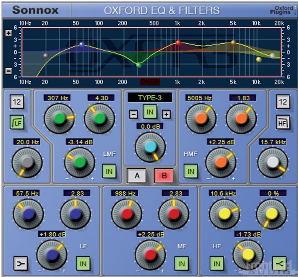
Figure 2.9. The basic EQ plug-in used by P6. It is seven-band parametric EQ where each of the seven filters is controllable by a set of knobs and button in the bottom portion while the shape of the overall frequency response curve is shown at the top. Dragging the circles on the graph at the top moves the corresponding knobs below.
