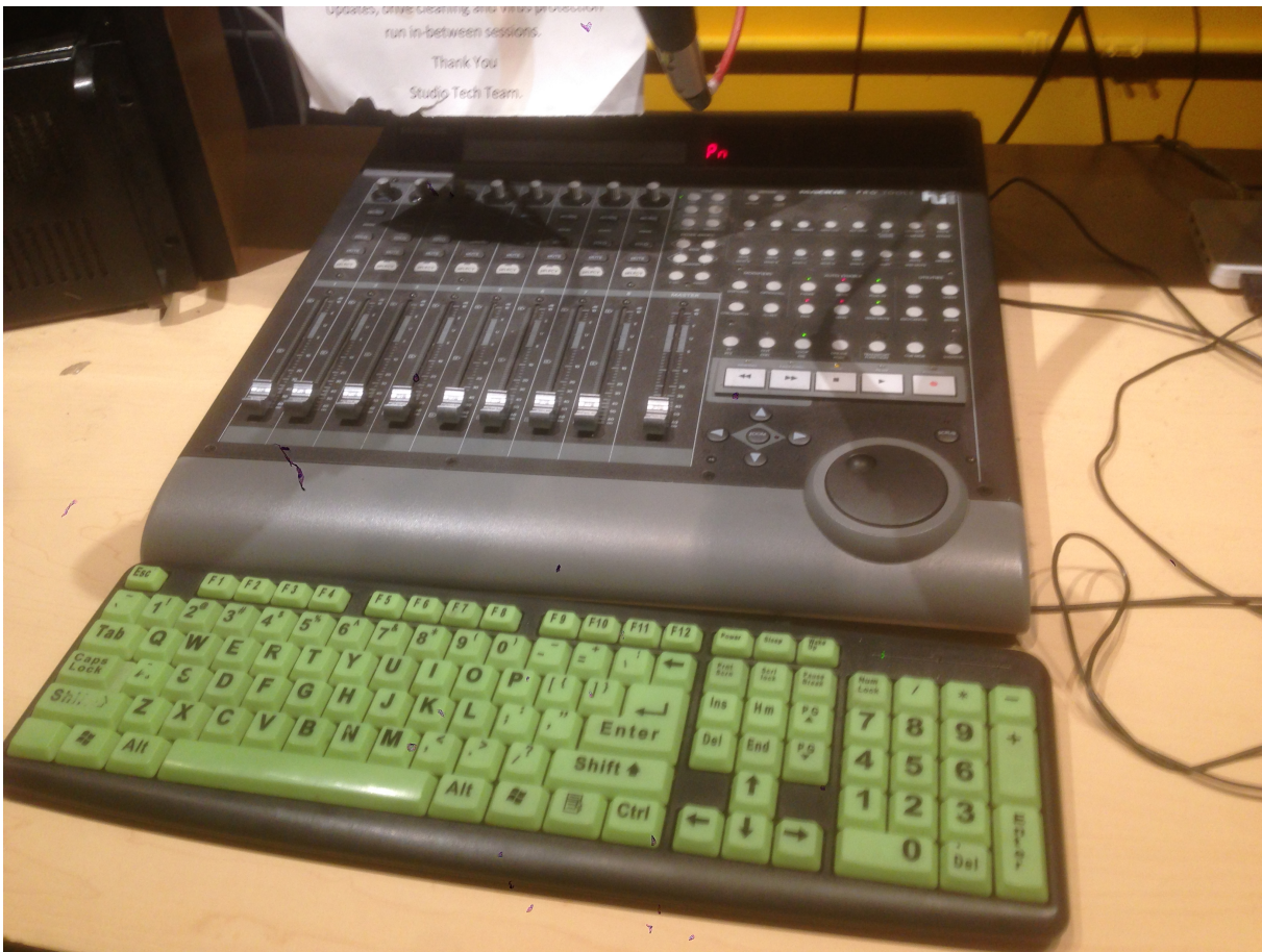
Figure 2.11. A control surface is a small mix suite in P2's studio. Unlike a mixing console, so audio passes through a control surface; it functions as a glorified keyboard/mouse for a DAW.
