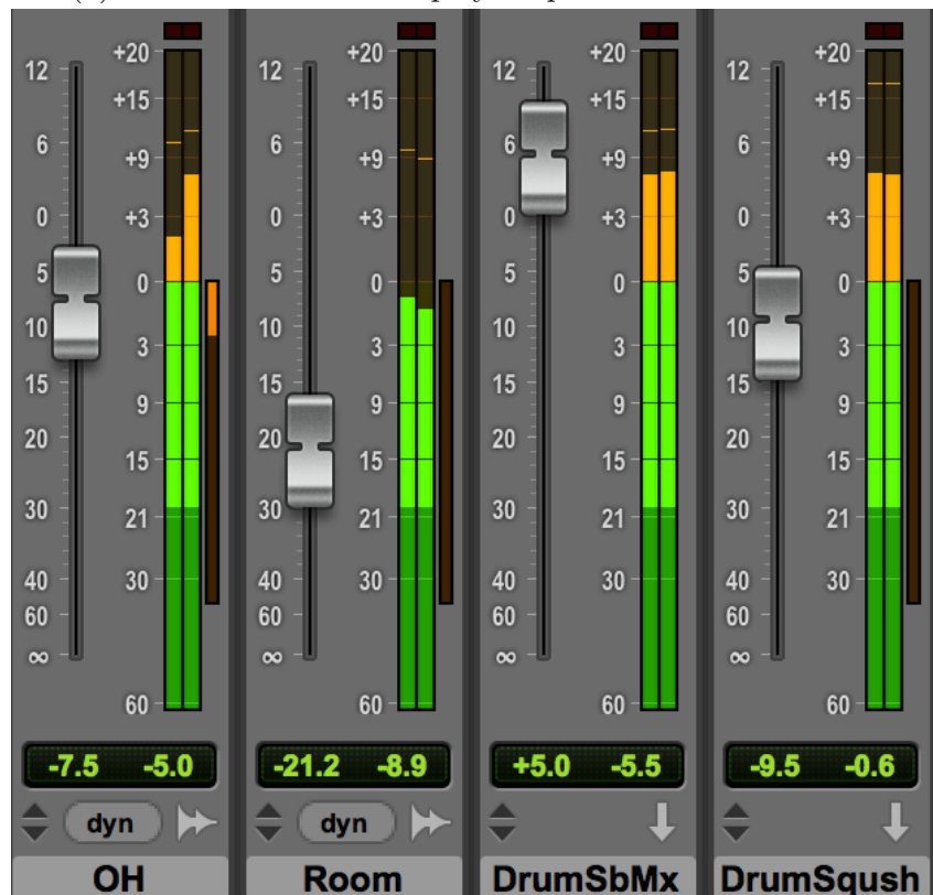
(b) Meters next to the faders in the Pro Tools mix window
