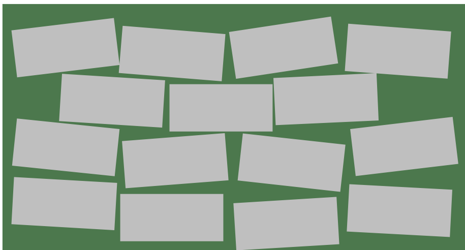
Figure 1 Mosaic model of a crystal. The tilting of the mosaic domains is exaggerated for clarity.
