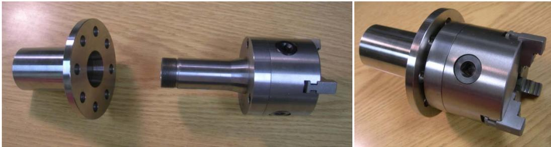
Figure 5.9 Photos of the 3-jaw chuck system.
