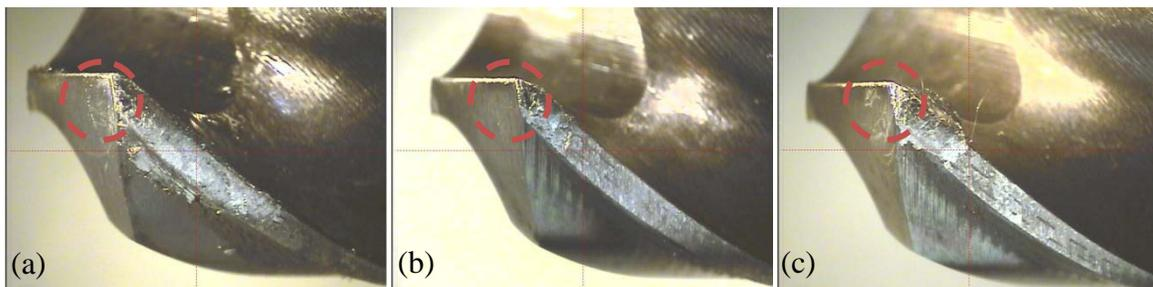
Figure 5.25 10% textured drills at failure (a) #1 after 45 holes drilled, (b) #2 after 60 holes drilled, and (c) #3 after 60 holes drilled. Circles indicate the tips of the drill bit margin where no textures were made.
