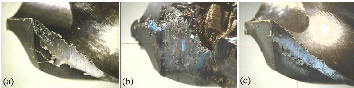
Figure 5.24 Baseline drills at failure (a) #1 after 30 holes drilled, (b) #2 after 52 holes drilled, and (c) #3 after 60 holes drilled.
