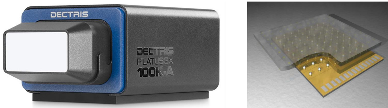
Figure 3.9 Photo of PILATUS 100K (left) ( 487 \times 195 = 94\,965 pixels with 172 \times 172 \mu\text{m}^2 for each pixel) and schematic of hybrid pixel array (right).
