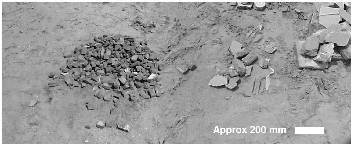
Figure 7.7 Small fragments not recorded, Frangible wall left, Conventional wall right.
