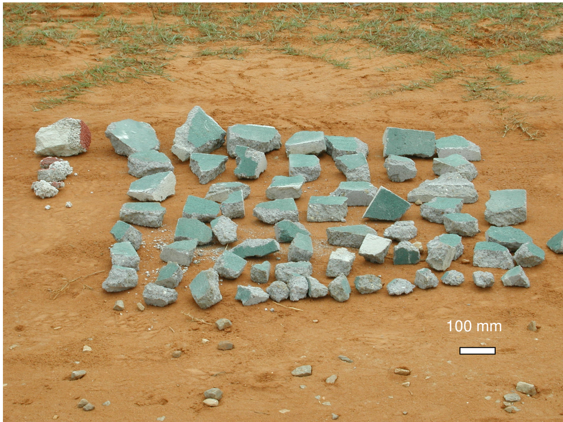
Figure 7.12 Photograph of the 70 pieces collected from the blast
