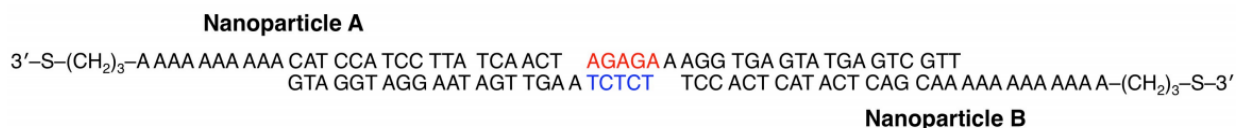
Figure 81. Hybridization between complementary linker strands leads to superlattice formation. The above schematic shows the design implemented for this work.
