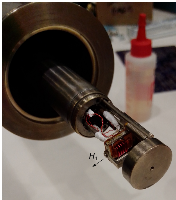
Figure 3.1. The sample stage and coil used in our high-field experiments at NHMFL. The direction of the H_1 field is indicated by the arrow and the label. The H_o field is perpendicular to H_1 and runs parallel to the axis of the of the probe.
