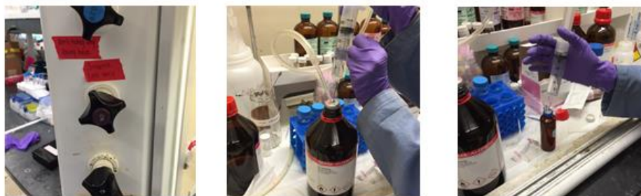
Figure A4.9: Diluting the phosphoramidites: (Left) The N 2 supply valve for the Schlenk line (Center) Drawing out Anhydrous ACN by piercing septum with long needle (Right) Adding ACN to the vented phosphoramidite bottles.
