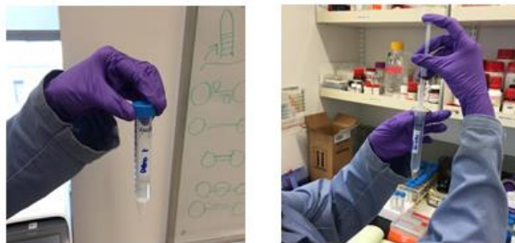
Figure A4.13: (Left) Centrifuged DNA-Water-CPG mixture showing separated CPGs at the bottom and DNA at the top. (Right) Syringe filtering the supernatant.
