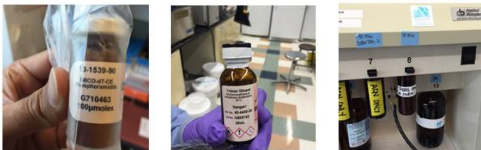
Figure A4.11: The DBCO phosphoramidite pack (left) and diluent (center). (Right) DBCO placed in a small glass tube inside an empty bottle and mounted on port 8 and CSO oxidizer mounted on port 15.
