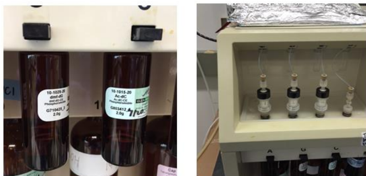
Figure A4.10: (Left) Phosphoramidite bottles loaded onto synthesizer using the black tab buttons. (Right) CPG filled columns affixed onto the synthesizer – reagents flow into the column from the bottom and come out through the tubing on the top.
