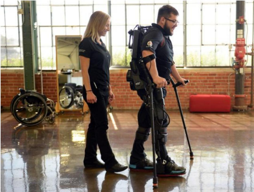
Figure 6.3. Ekso Bionics exoskeleton, EksoGT™, used for data collection. We use two sets of its sensors in this study: hip and knee encoders to generate kinematics-based dynamical models using the NCD algorithm, and foot-mounted pressure sensors at the heel and toe to validate our models against ground-contact events after partitioning.
