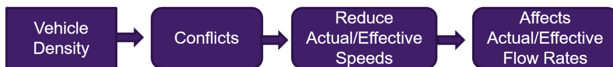
Figure 4.1. The process by which aircraft density in a given airspace affects the traffic flow of aircraft.
