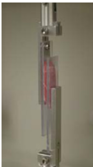
Figure 4.6 Testing apparatus, arranged for longitudinal shear, for direct measurement of shear modulus. Image from Morrow et al. (2010)
