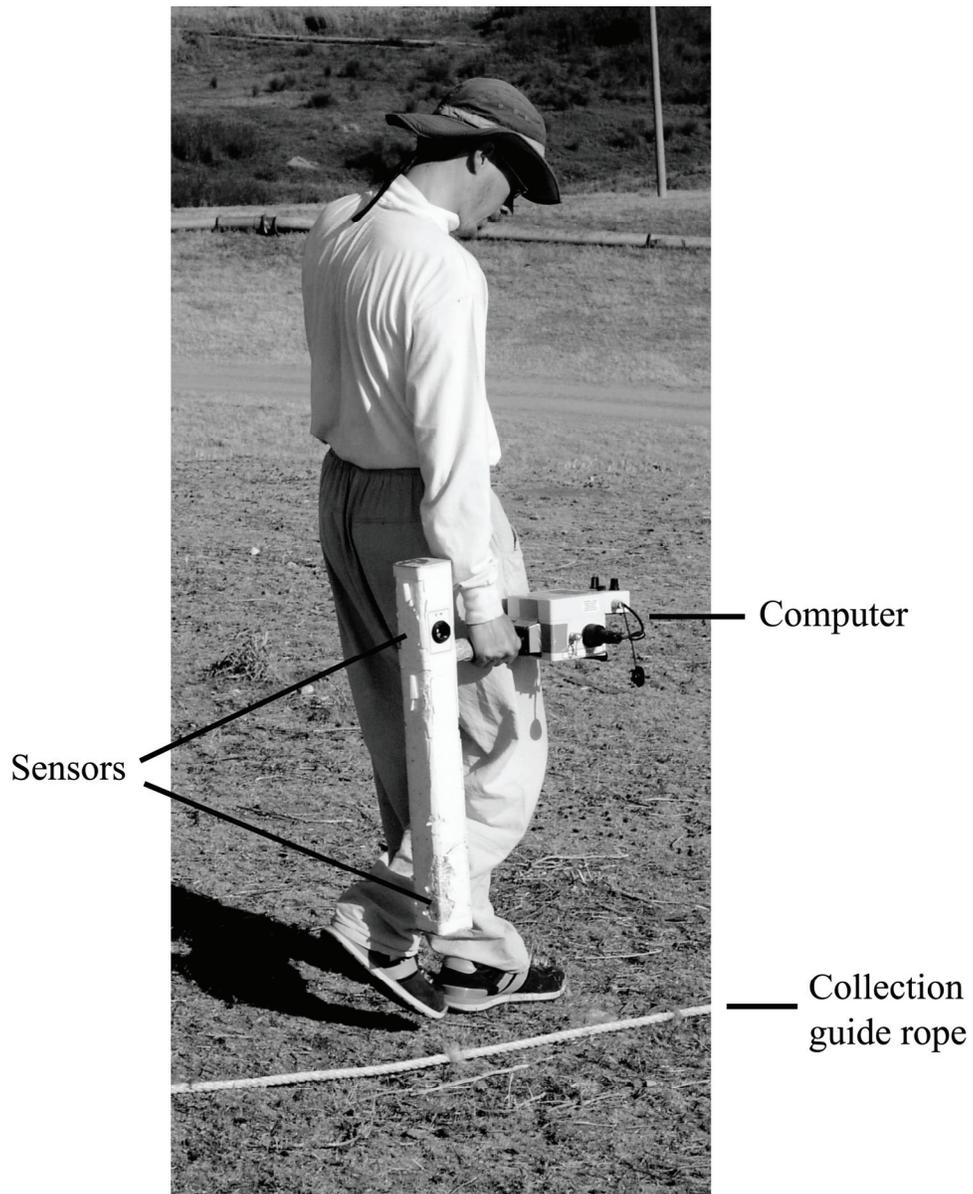
Figure 4.1: The FM 36 Gradiometer in use.
