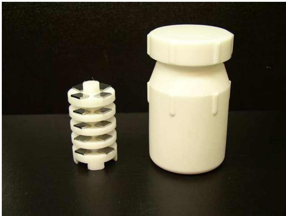
Figure 3.1 Image of the Teflon© air tight container and matching custom made sample holder used to vapor deposit silane onto NiTi.
