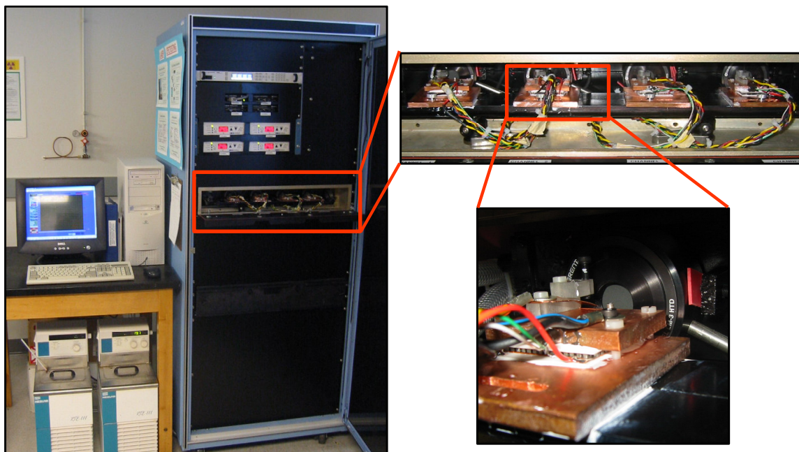
Figure 6.2 – QCL lifetime and reliability testing system at the Center for Quantum Devices
