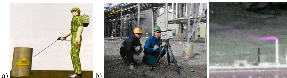
Figure 1.3 – (a) Example of optical remote sensing in a military application, similar to the L-PAS system under development by DARPA. (b) Example of optical remote industrial chemical and pollution monitoring.
