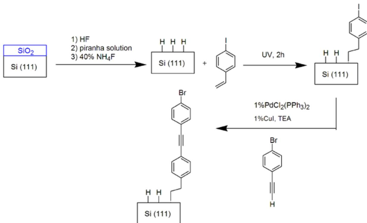
Figure 4: Synthetic scheme for solid phase Sonogashira coupling.
