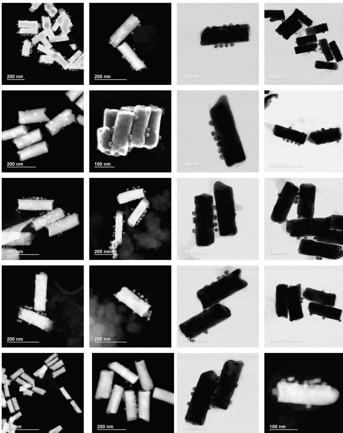
Figure A.1. Additional STEM micrographs for the directed assemblies of 20 nm Au nanoparticles onto the selectively functionalized barrels of Au nanorods.
