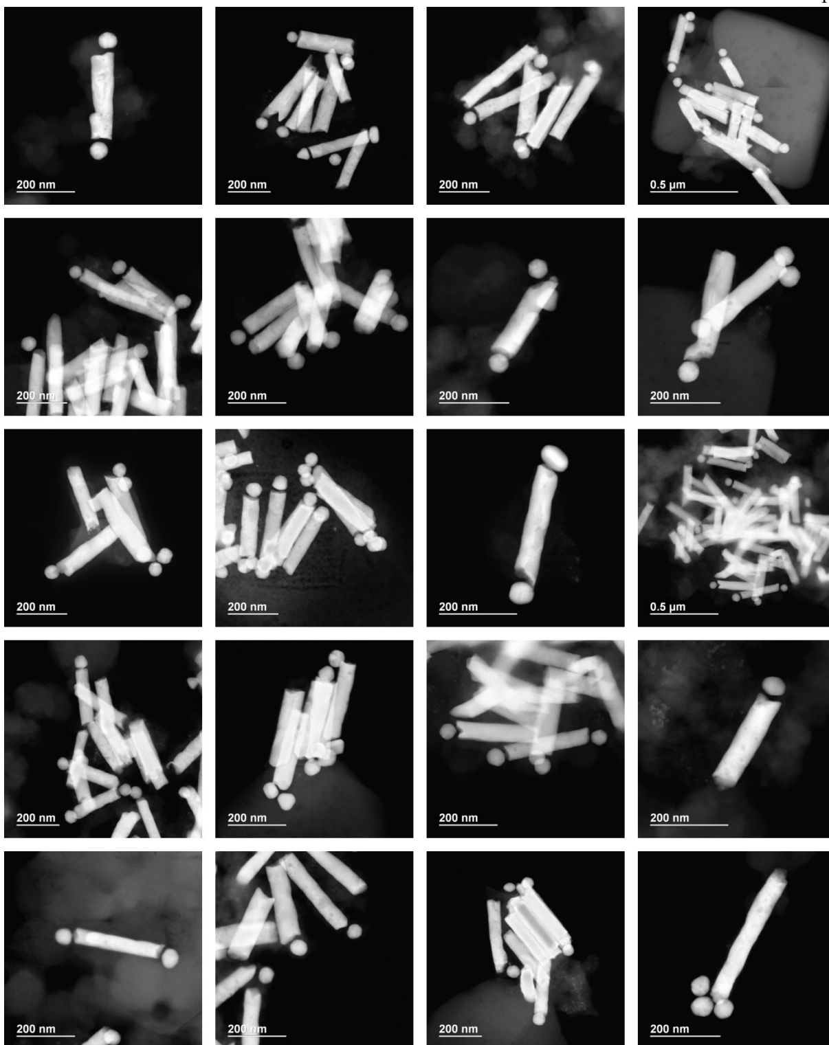
Figure A.5. Additional STEM micrographs for the directed assemblies of 60 nm Au nanoparticles onto the selectively functionalized bases of Au nanorods.
