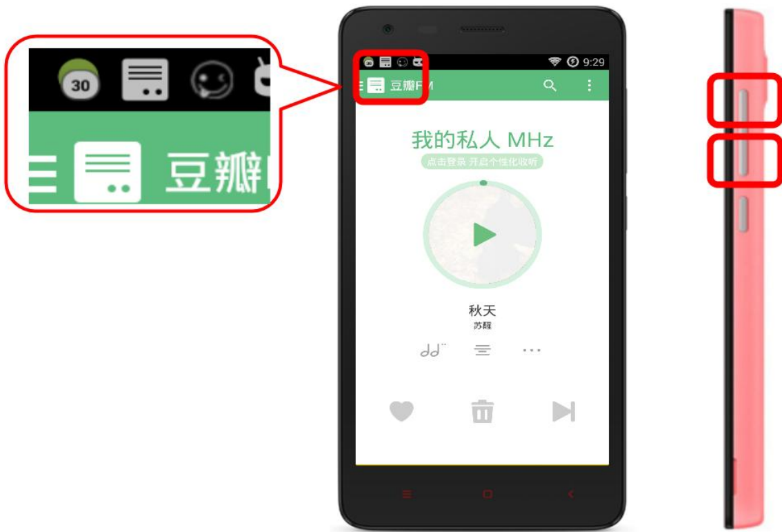
Figure 5.1: DelayController interface, which shows the user the current delay setting (30%), and allows the user to control the delay using the volume keys, shown over Kingsoft.
