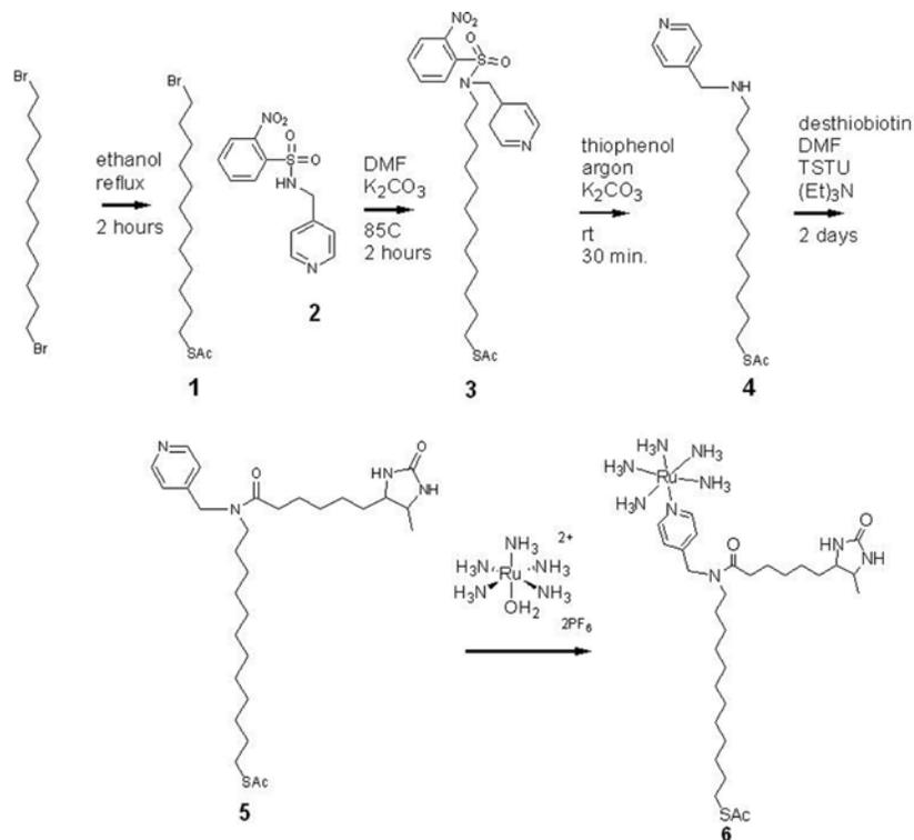
**Figure 3: Overall synthesis of the target redox-modified ligand. Ruthenium pentaamine is the redox modification, and desthiobiotin is available for binding to avidin. The thioacetate in 6 can be deprotected to give a thiol to attach to the gold electrode.**
