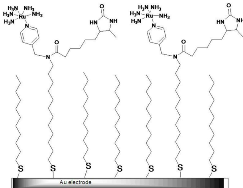
**Figure 2:** The target system incorporated into a monolayer on a gold electrode. Undecanethiols are placed in between the ligands to prevent other molecules in the solvent from transferring electrons to the electrode.
