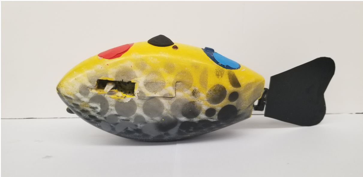
Figure 8.8. Tail-actuated robotic fish used in experiments, developed by the Smart Microsystems Lab at Michigan State University. It maneuvers in water by oscillating its tail fin.
