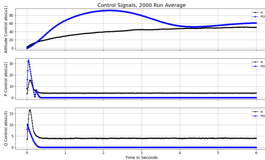
Figure 6.4: A comparison of AI vs Traditional PID control, looking specifically at the signal output of both systems. Time averaged over 2000 runs with different initial conditions.
