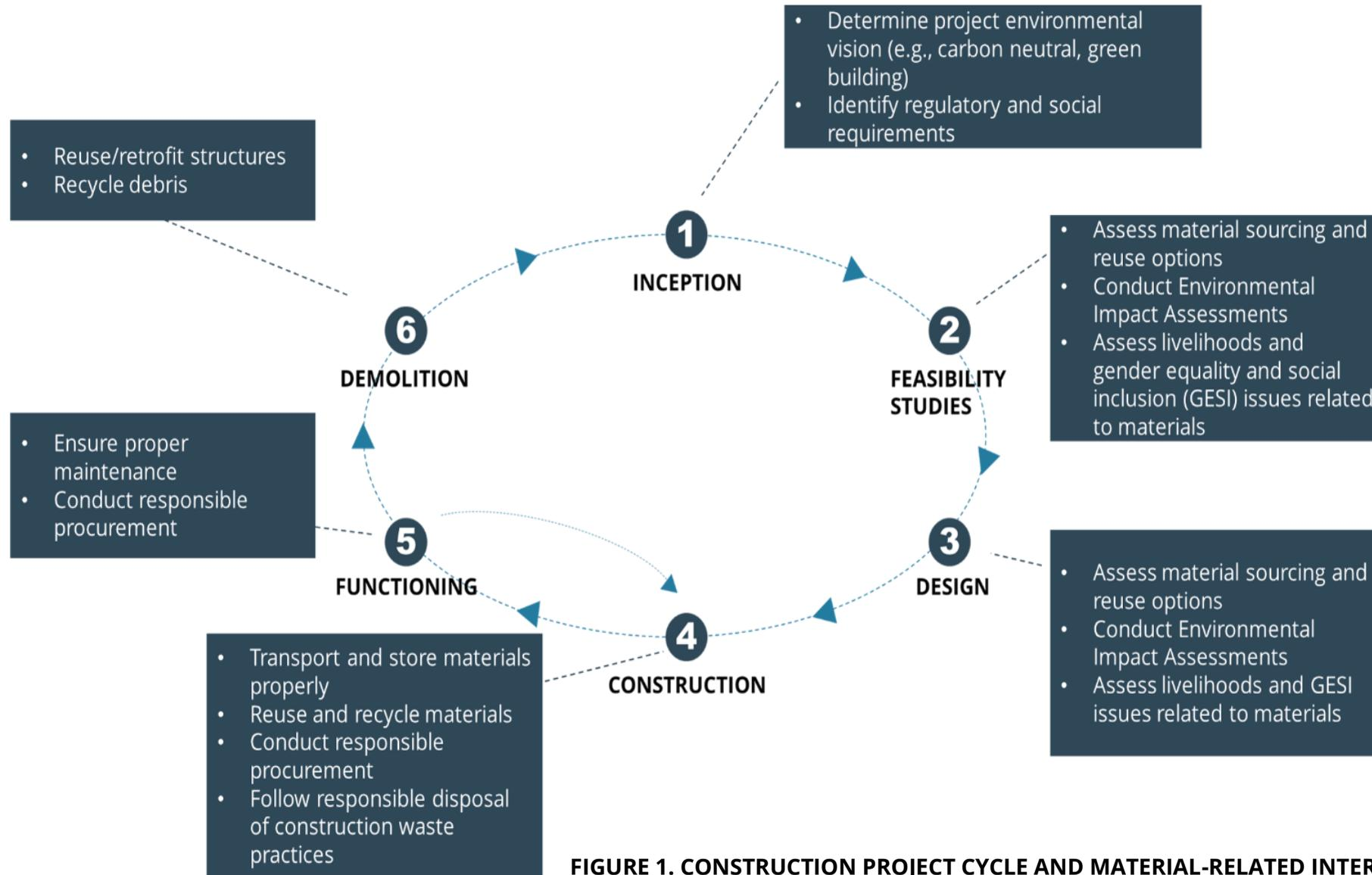
**FIGURE 1. CONSTRUCTION PROJECT CYCLE AND MATERIAL-RELATED INTERVENTION POINTS**
