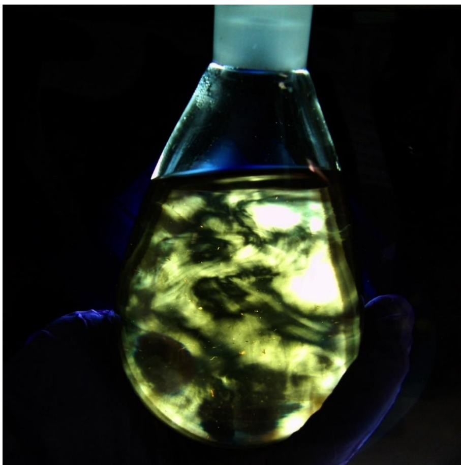
Figure 2.5. Optical schlieren are observed from dilute GO in a large acetone bath. GO sheets precipitated to the bottom of the bath, but could be briefly redispersed by swirling. When this solution is photographed between crossed polarizers, light and dark bands are seen, indicating the presence of orientationally-ordered domains.
