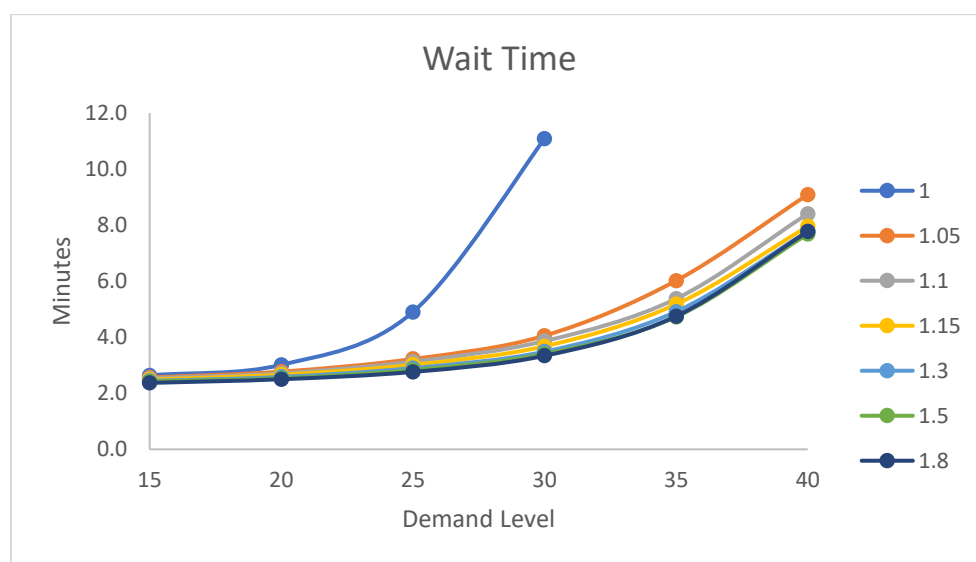
Figure 7-2: Average user wait time as a function of demand (x-axis) and maximum user detour time/distance (line color)
