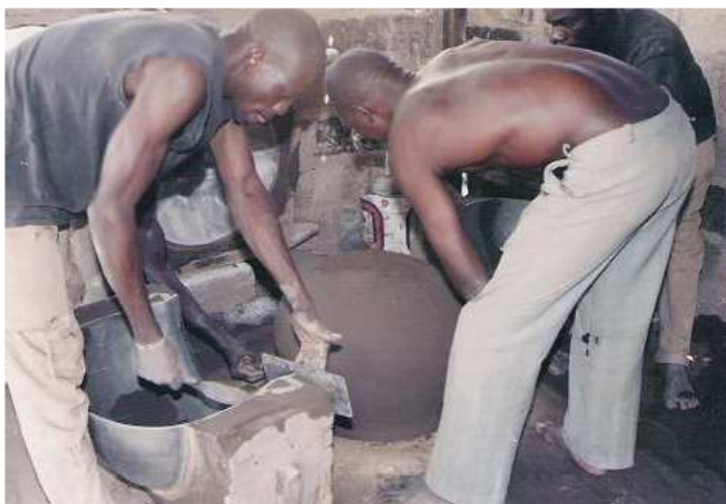
Photo 41 and 42. Philippe sprinkling additional sand on the bottom of the mold.
