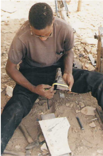
Photo 63. Taking the dimensions of the original seat.
