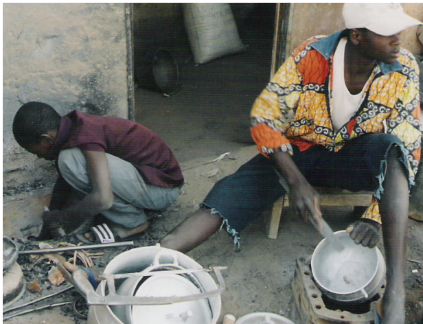
Photo 37. Apprentice (right) filing imperfections off the castings.
