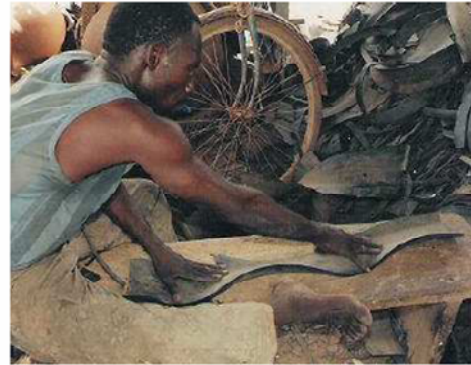
Photo 88. Laying the strip before drawing the soles.
