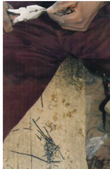
Photo 111. Folding and cutting staples with a pair of pliers.
