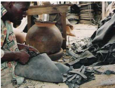
Photo 107. Cutting thin strips of inner-tube to make a spiral around the thong.
