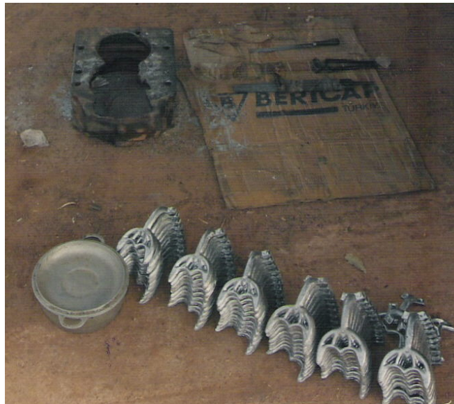
Photo 129. Series of ceiling fan parts that have already been cast and polished.
