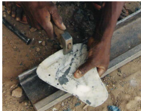
Photo 68. Shaping the back of the seat.
