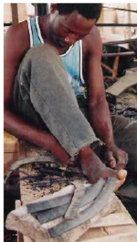
Photo 101. Cutting straps out of the strip of "bante." The first one is used as a pattern for the others, in order for all of them to have the same dimensions.
