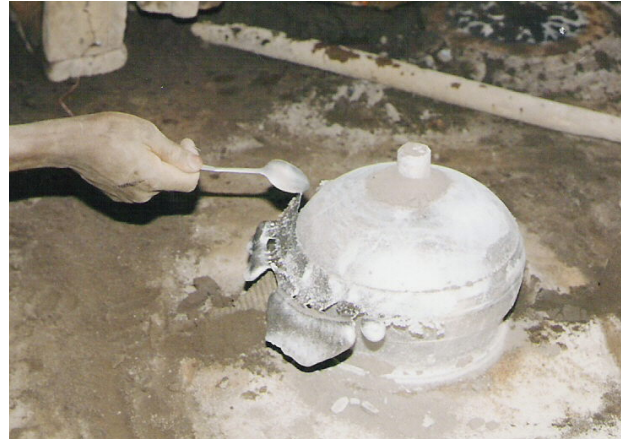
Photo 36. Failed pot: they did not press hard enough and some aluminum leaked out.
