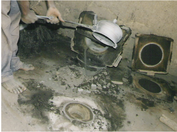
Photo 35. Taking the casting out of its mold.
