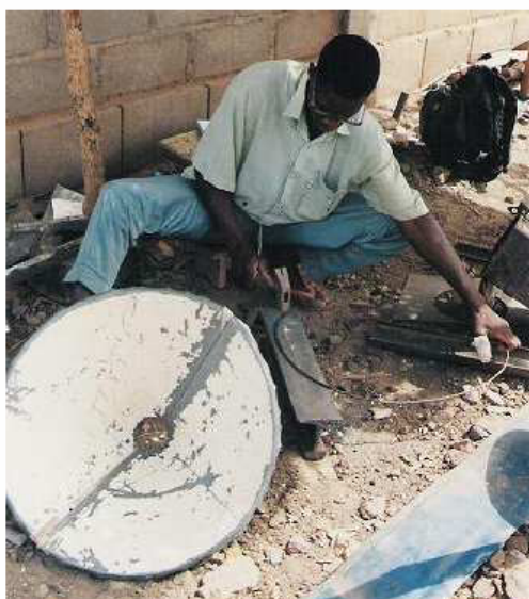
Photo 57. Bending the iron wire to fit the shape of the funnel.
