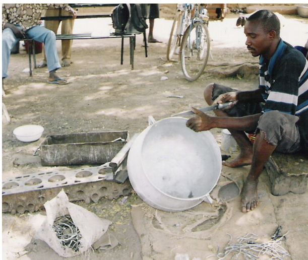
Photo 39 & 40. Filing the castings and plugging any holes.
