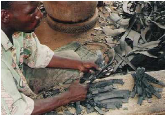
Photo 103. Cutting one end of each strap to make it round.
