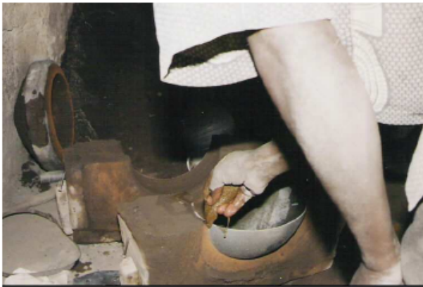
Photo 23. Wetting the handles before removing the metal mold.
