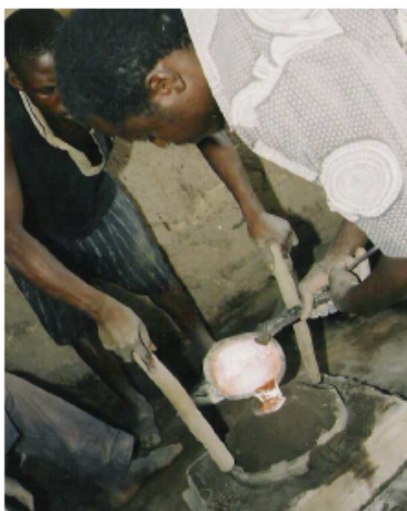
Photo 31. Carefully placing the sapo back on top of the bottom frame, making sure that the marks that had been made fit correctly in their exact position.
