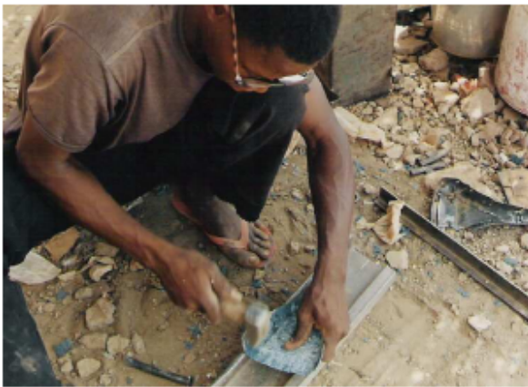
Photo 69. Shaping the sides.
