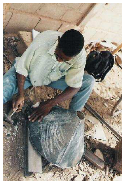
Photo 58. Folding the top edge over the wire.
