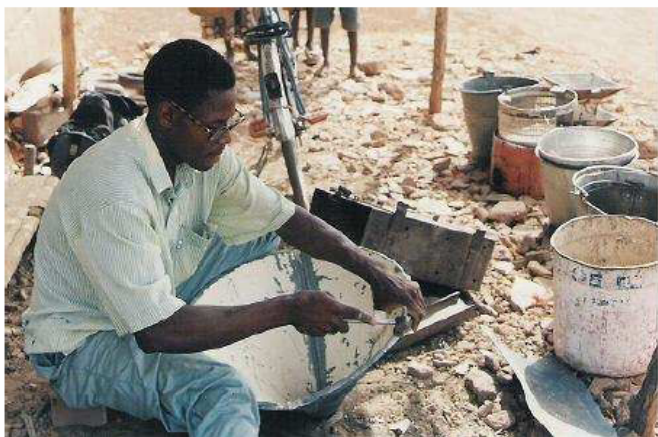
Photo 55. Hammering the top edge outwardly.
