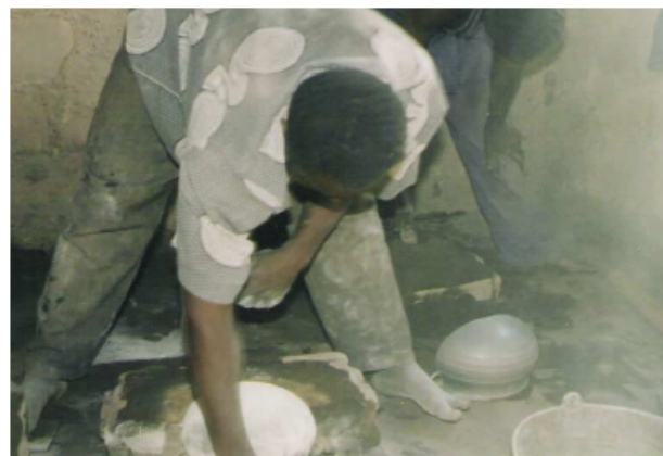
Photo 28. Placed one half of the sand mold back and smoothing the inside section with the back of a spoon.
