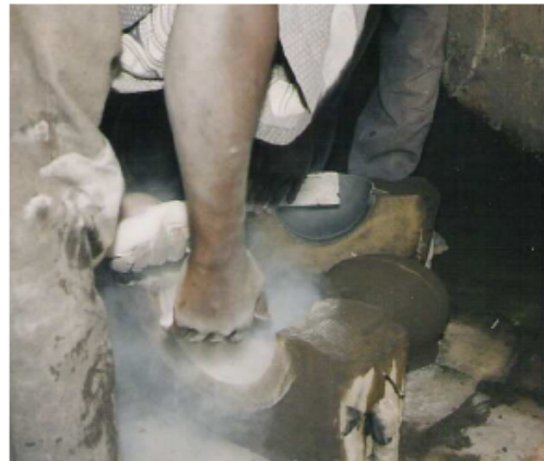
Photo 24. Spreading a type of powdered clay ( go:re ) after smoothing the side of the sand mold.
