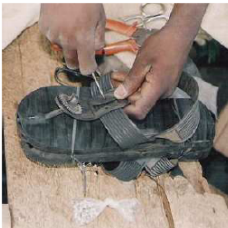
Photo 125. Piercing a hole in the upper with a needle.
