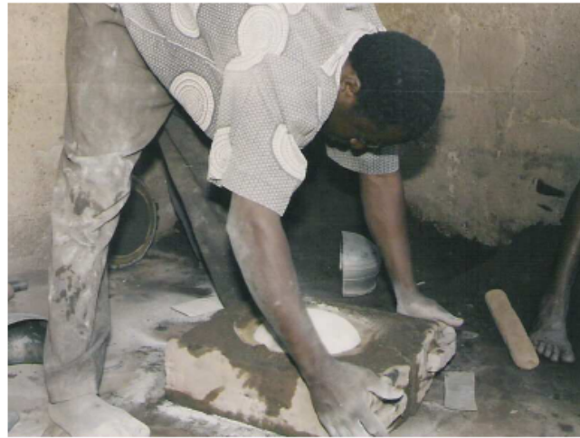
Photo 30. Placing the second half of the bottom frame back around the inside section. Checking the space between the outer and inner molds and pressing the frames to adjust it.
