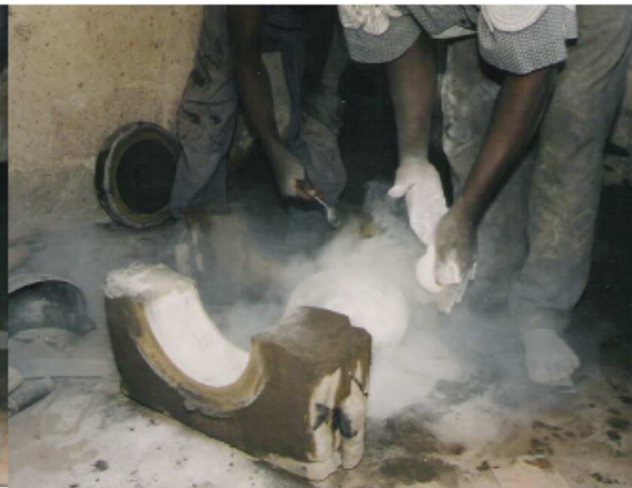
Photo 26. Spreading go:re on the inside section of the sand mold.
