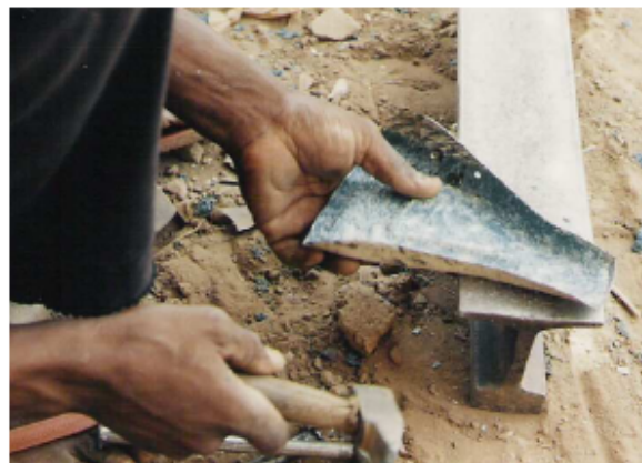
Photo 70. Bending the sides.
