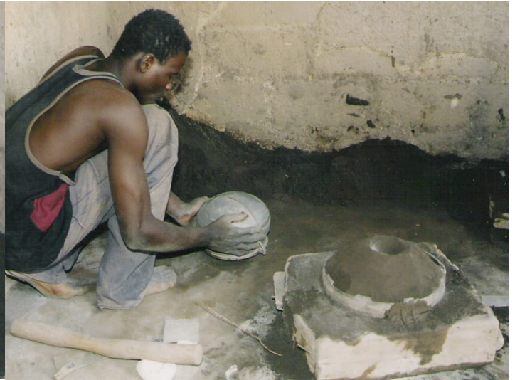
Photo 9. Tying the two halves of the mold with a metal belt and a wooden wedge.
