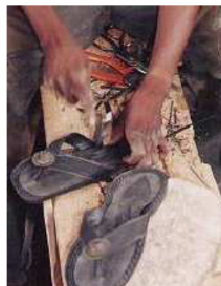
Photo 115. Stapling the sides of the straps into the side-slots of the sole.
