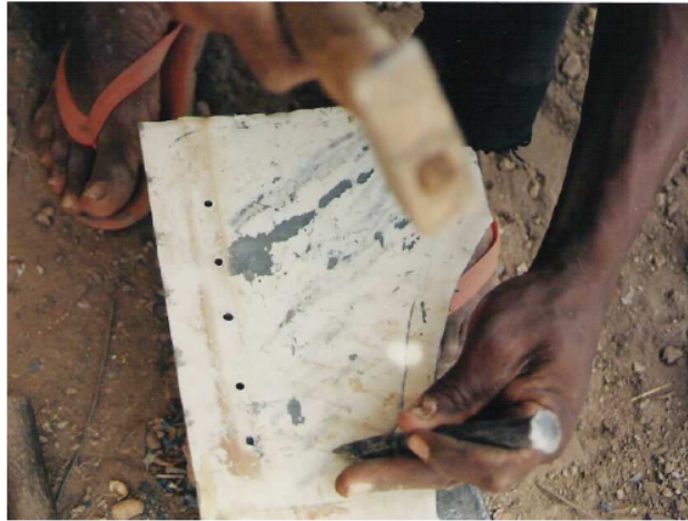
Photo 64. Cutting the outline of the original pattern after having marked it.
