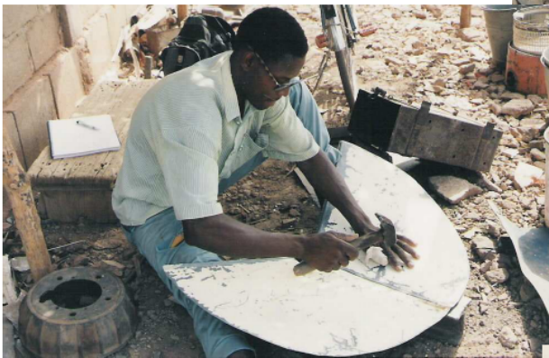
Photo 53. Fixing the two sides together, hammering on the seam.
