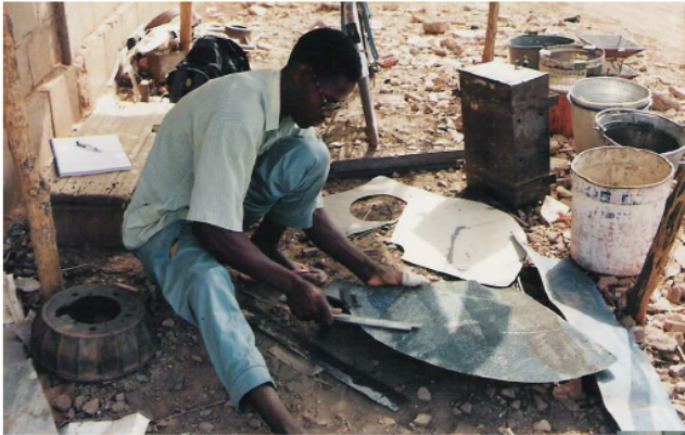
Photo 51. Flattening the sheet with a päbgha (a thin, flexible metal slat)
