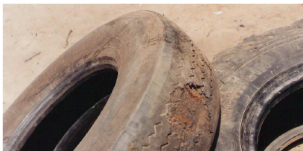
Photo 75. Used tire: the bead has been removed, as well as the tread (left) and the sidewalls.
