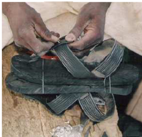
Photo 126. Placing the lower part of a decorative snap fastener ( rivet ) underneath the upper.
