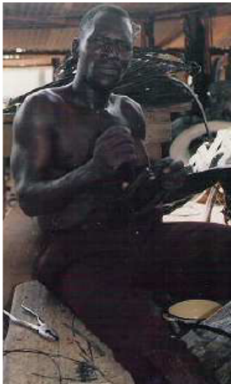
Photo 110. Unfolding a roll of wire (tire bead) to make staples.
