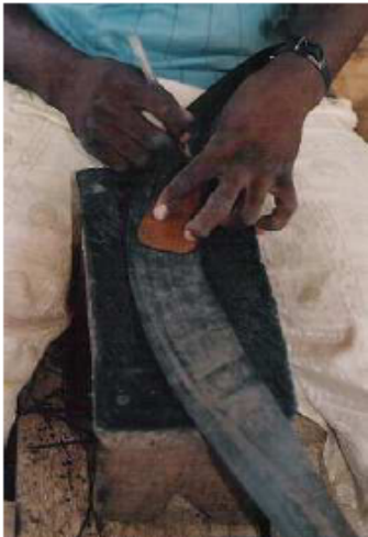
Photo 117. Drawing the pattern of the upper onto a strip of "bante."
