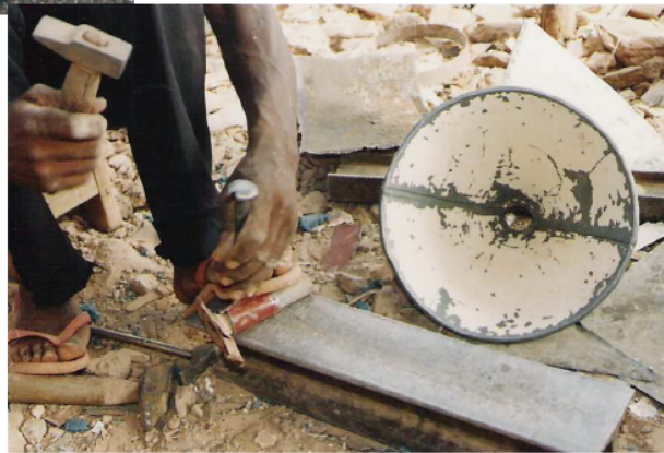
Photo 60. Making a tube that will be fixed at the bottom of the funnel.
