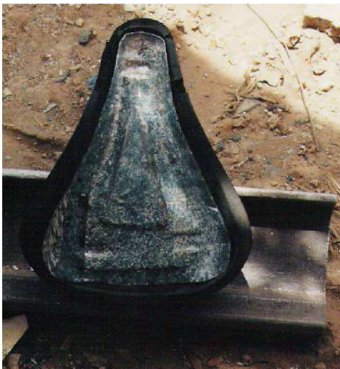
Photo 74. Finished seat. There only remains to make two holes in the front of the seat in order to screw it on the bicycle.
