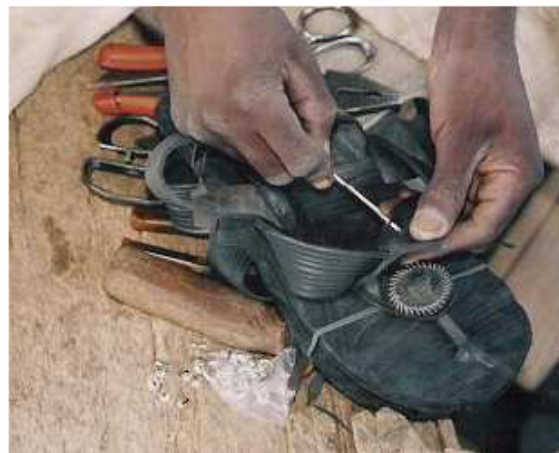
Photo 126. Placing the lower part of a decorative snap fastener ( rivet ) underneath the upper.
