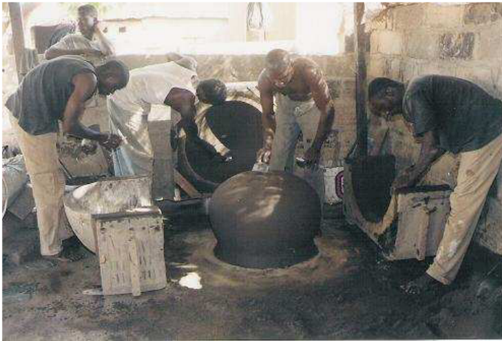
Photo 44 and 45. Smoothing the additional sand with a spatula, until it is completely integrated into the sand mold.
