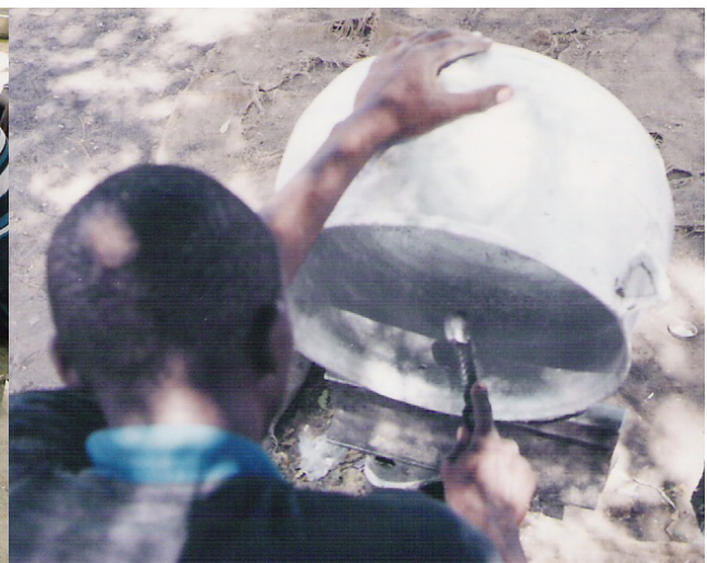
Photo 39 & 40. Filing the castings and plugging any holes.
