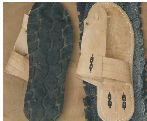
Photo 83. Piece of tire tread added on the soles of leather sandals.
