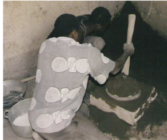
Photo 19. Boss taking over, placing a metal tube ( sprue ) in the middle (in contact with the metal mold underneath) and ramming the sand around it to make it firm.
