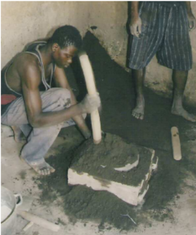
Photo 18. Added the top frame ( sapo ), filled it with sand and ramming it clockwise.
