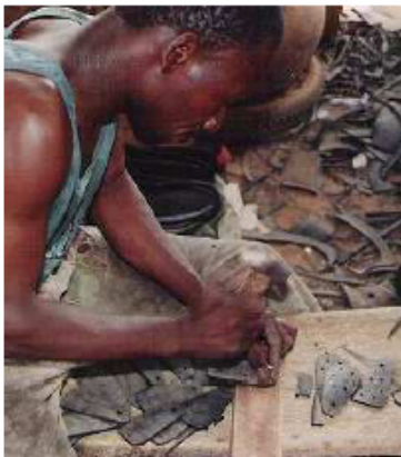
Photo 120. Making holes in the uppers, using an inner-tube valve.
