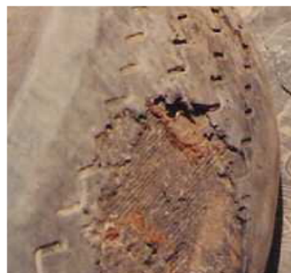
Photo 76. Damaged bias-ply tire ( gisga pneu ): we can see the nylon threads coming out.
