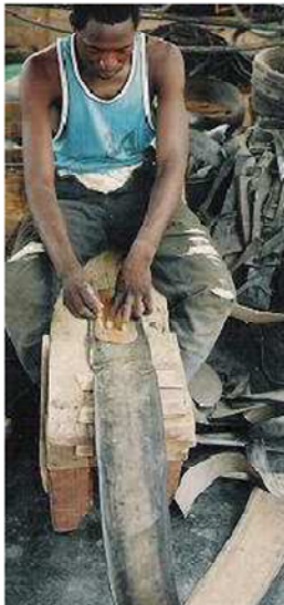
Photo 89. Tracing the outline of the pattern
