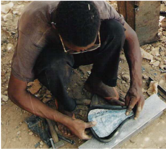
Photo 71. Placing the new seat in the seat cover to see if it fits and checking what needs to be improved.
