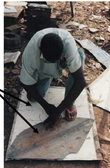
Photo 48. Changed the position of the pattern to be able to draw both sides of the funnel on one sheet.
