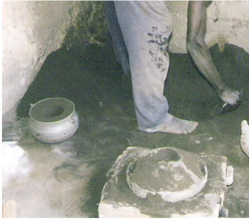
Photo 12. Made a hole in the sand on top of the mold (left).
