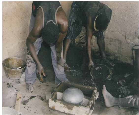
Photo 15. Tying the two halves of the wooden bottom frame ( ruk rogo ) together and placing the two metal plates.
