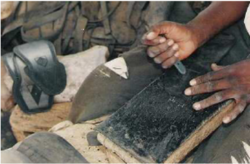
Photo 95. Carving the designs on the sole.
