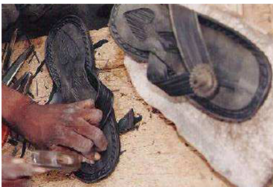
Photo 114. Stapling the thong into the front slot of the sole.
