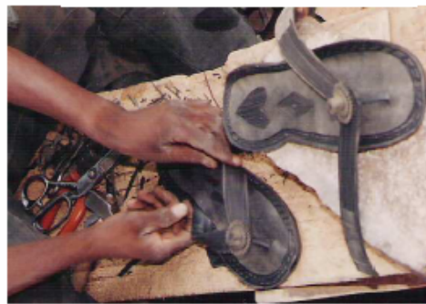
Photo 113. Placing the straps into the side-slots.
