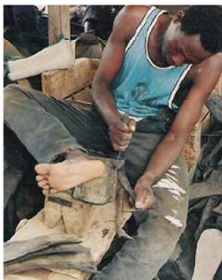
Photo 92. Cutting the sole out of the "bante"
