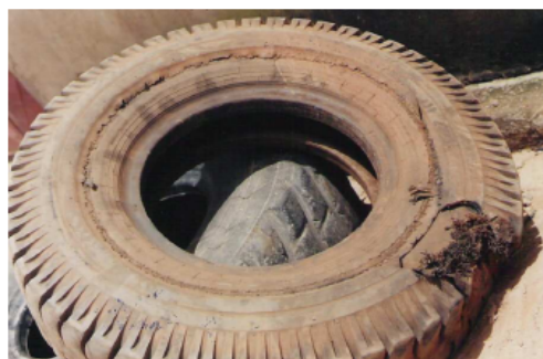
Photo 76. Damaged bias-ply tire ( gisga pneu ): we can see the nylon threads coming out.
