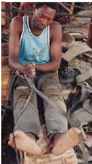
Photo 100. Cutting the "bante" in its length.
