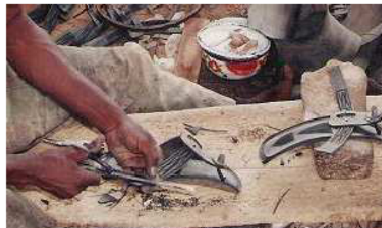
Photo 123. Adjusting the length of the straps before sliding them into the side-slots of the soles.
