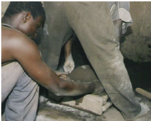
Photo 31. Carefully placing the sapo back on top of the bottom frame, making sure that the marks that had been made fit correctly in their exact position.
