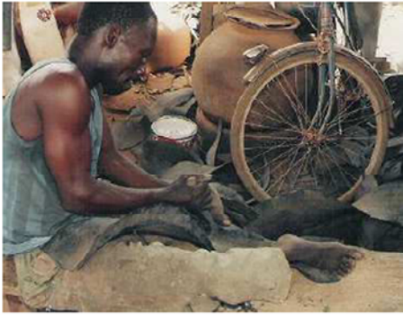
Photo 87. Cutting the uneven edges of a strip of «bante» (inner liner)
