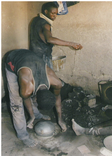
Photo 14. Turning the mold upside down and making sure it is tight.
