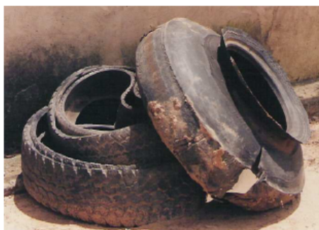
Photo 75. Used tire: the bead has been removed, as well as the tread (left) and the sidewalls.
