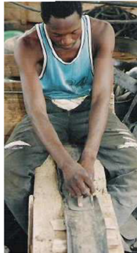
Photo 90. Tracing the other side of the pattern
