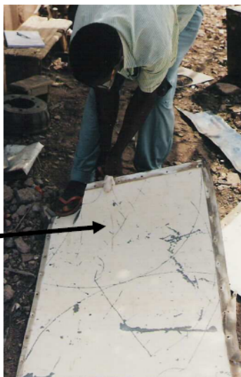
Photo 49. Beginning to cut the pattern with snips.
