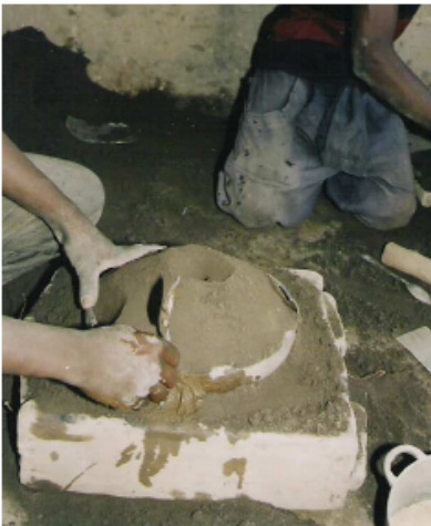
Photo 20. Wetting the sand on both sides to mark the emplacement of the sapo on top of the bottom frame ( ruk rogo ).
