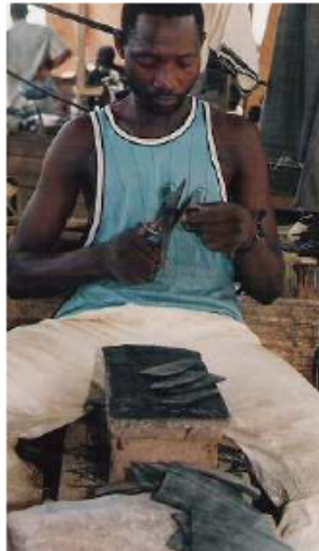
Photo 118. Cutting the uppers with scissors.
