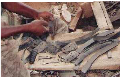
Photo 122. Sliding the straps into the slots of the uppers.
