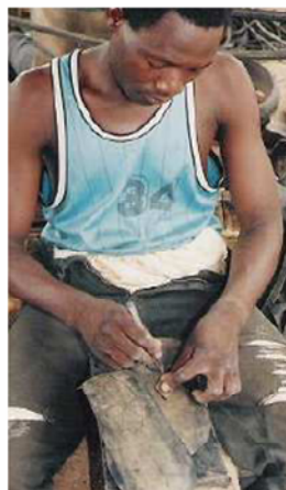
Photo 93. Drawing the shape of the patterns on the sole (decoration).
