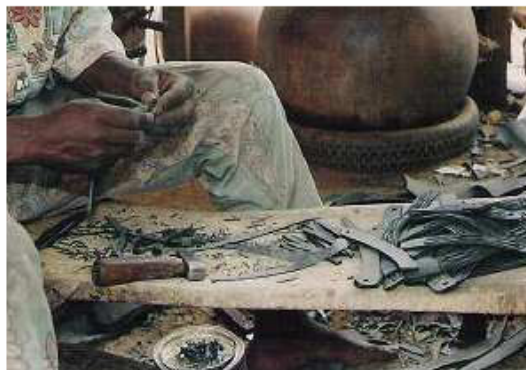
Photo 108. Rolling the inner-tube strip around each thong ( yôr bāngā ) to make a spiral. The thongs are pieces of "bante" that were already prepared before starting this series of sandals.
