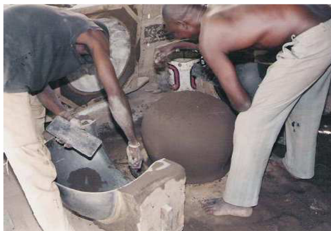
Photo 41 and 42. Philippe sprinkling additional sand on the bottom of the mold.
