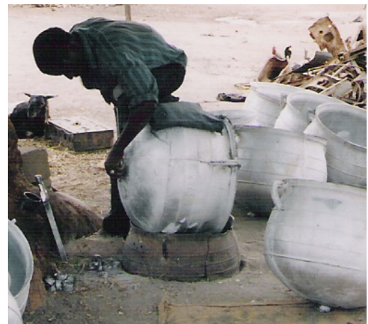
Photo 38. Sawing the tips (sprues) of the castings.
