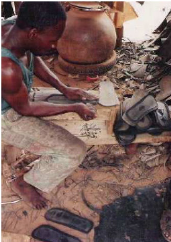
Photo 97. Cutting a slot on each side of the sole, near the back, where the straps will fit
