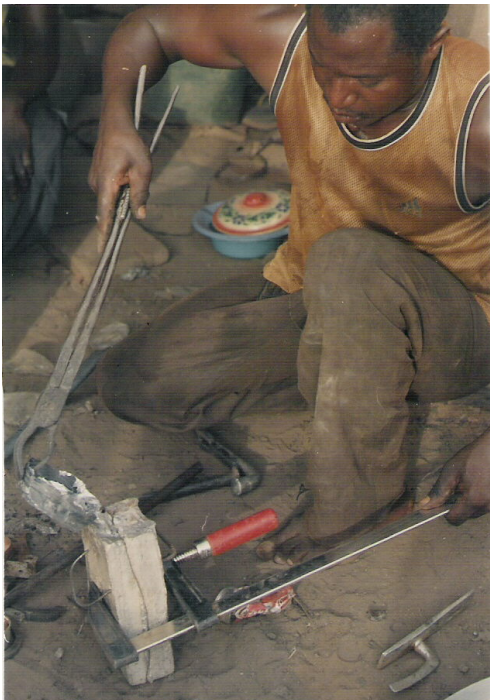
Photo 128. Paul pouring aluminum into the mold that was specially created for the purpose of this order of ceiling fan parts.
