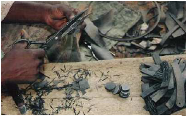
Photo 105. Cutting a series of circles out of the "bante."
