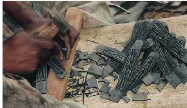
Photo 104. Making a hole in the rounded end of each strap, where the thong will go through. Boureima uses an inner-tube valve to do so.
