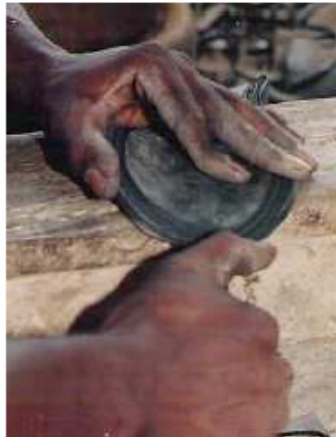
Photo 98. Cutting a slot in thickness of the sole, on the front. The blade pushes in until it reaches the slot that was previously cut on the front of the sole (making a way for the thing).
