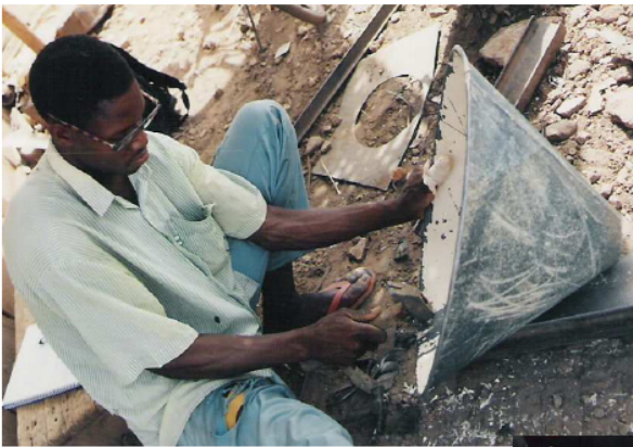
Photo 59. Hammering the edge to wrap the wire.
