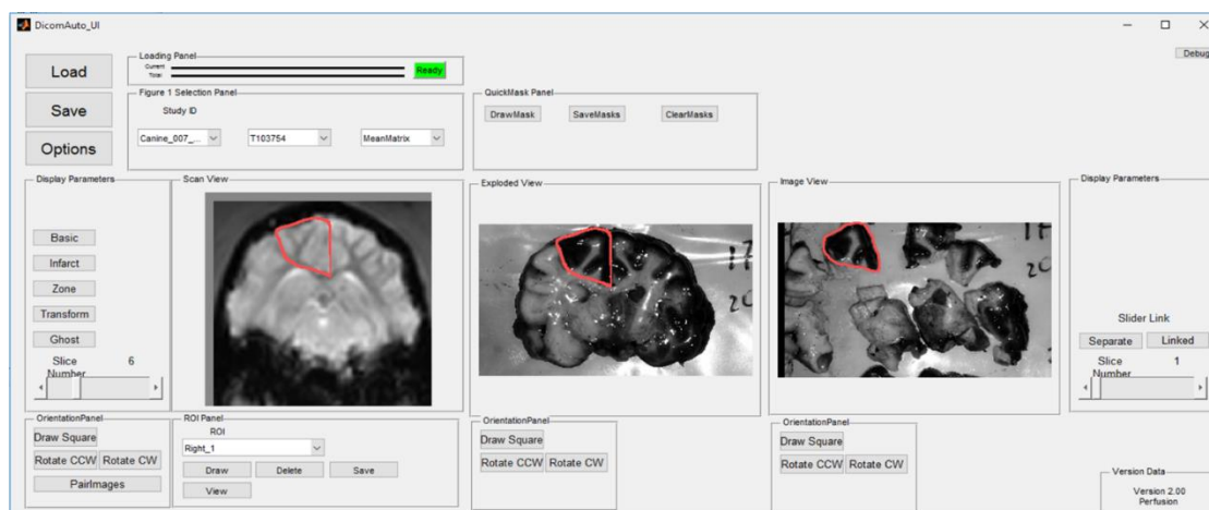
Figure 5.3: Screenshot from Graphical User Interface. Screen shot from the graphical user interface developed to allow for registration of microsphere laden tissue samples to the MRI perfusion images.
