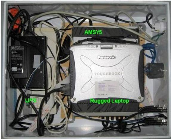
(a) Interior of enclosure showing AE unit, rugged laptop, and battery-backed power supply
