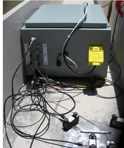
(b) AE enclosure deployed on the top chord of the Kennedy Bridge
