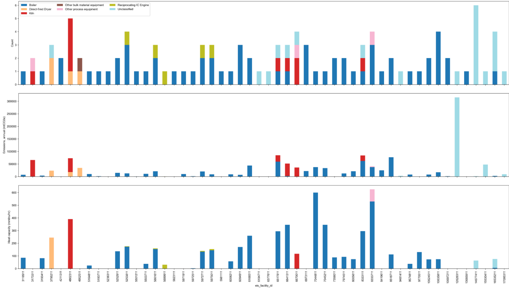
Figure C-0-4. Distribution of unit types by total number of units, GHG emissions, and total capacity for individual facilities in the Sawmills industry (321113) from NEI data
