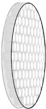
**Figure 1:** Idealized representation of a microporous thin film with uniform thickness and a well-defined porous structure.
