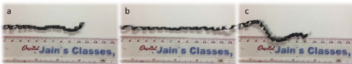
Figure 3.12. A flexible and stretchable GO coil spring.
