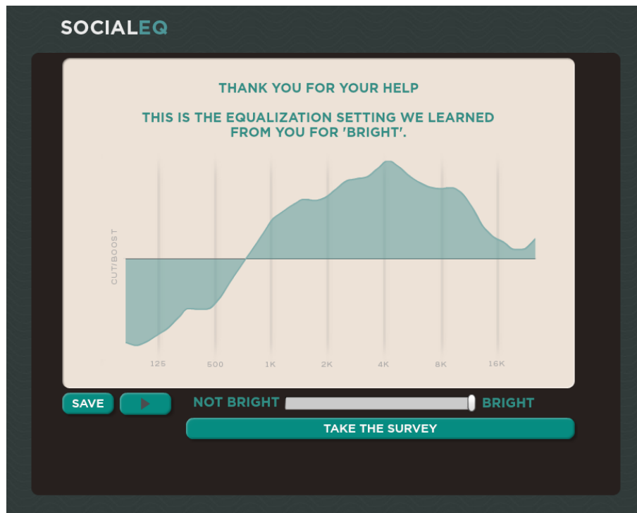
Figure 2.4. The equalization curve and control slider learned for “bright” in a single session.
